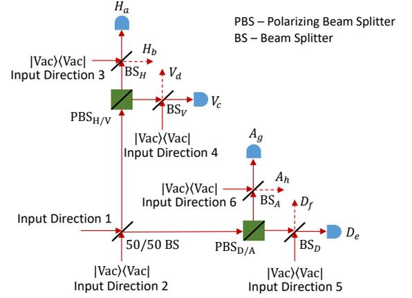
FIG. 16: Description of the measurement under the passive-detection scheme. Suppose that the detection efficiencies associated with the outcomes  $H, V, D$  and  $A$  are  $\eta_H, \eta_V, \eta_D$  and  $\eta_A$  respectively, and that the four detectors shown are ideal. Then, the beam splitters  $BS_H, BS_V, BS_D$  and  $BS_A$  have transmission coefficients  $\sqrt{\eta_H}, \sqrt{\eta_V}, \sqrt{\eta_D}$  and  $\sqrt{\eta_A}$ , respectively.
