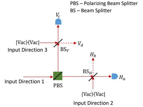
FIG. 15: Description of the measurement in the  $H/V$  basis under the active-detection scheme. Suppose that the detection efficiencies associated with the outcomes  $H$  and  $V$  are  $\eta_{H/D}$  and  $\eta_{V/A}$ , respectively, and that the two detectors shown are ideal. Then, the beam splitters  $BS_H$  and  $BS_V$  have transmission coefficients  $\sqrt{\eta_{H/D}}$  and  $\sqrt{\eta_{V/A}}$ , respectively.
