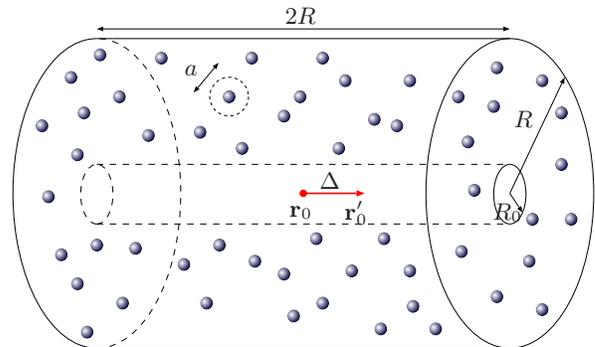
FIG. 1: Sketch of the system. The strongly scattering medium lies between two cylinders of radii  $R_0$  and  $R$ , respectively, and of length  $2R$ . The inner region with radius  $R_0$  corresponds to the region within the medium in which the fluorescent source is free to move, from position  $\mathbf{r}_0$  to position  $\mathbf{r}'_0$ . To mimic hard spheres correlations, a minimum distance  $a$  is forced between scatterers.
