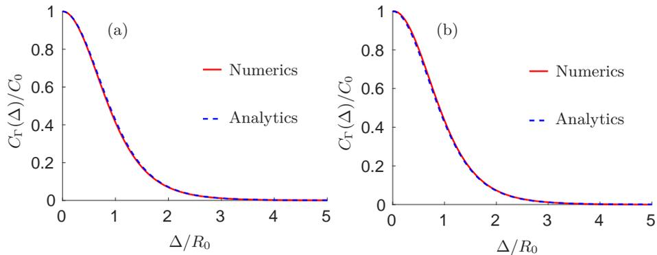
FIG. 3: Numerical (red solid line) and analytical (blue dotted line) spatial decay rate correlation  $C_r$  normalized by  $C_0$  as a function of the normalized distance  $\Delta/R_0$  for  $f = 1 \times 10^{-3}$  (a) and  $f = 0.1$  (b). Same parameters as in Fig. 2.
