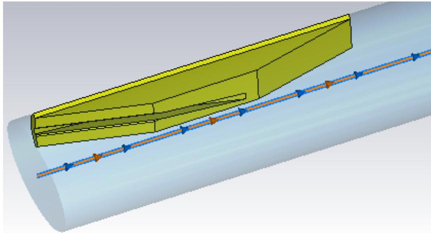
FIG. 14. Elliptic vacuum chamber with one absorber<sup>28</sup>.
