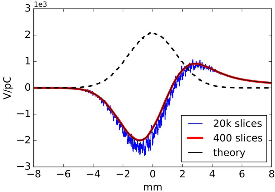
FIG. 7. Comparison of the analytical longitudinal wake potential of a 1.6 mm Gaussian bunch (black line) with those given by the simulation code, one using  $2 \times 10^4$  slices and the wake function as Green function (blue line), and the second one with 400 slices and the wake potential of a 0.15 mm Gaussian bunch as Green function (red line).
