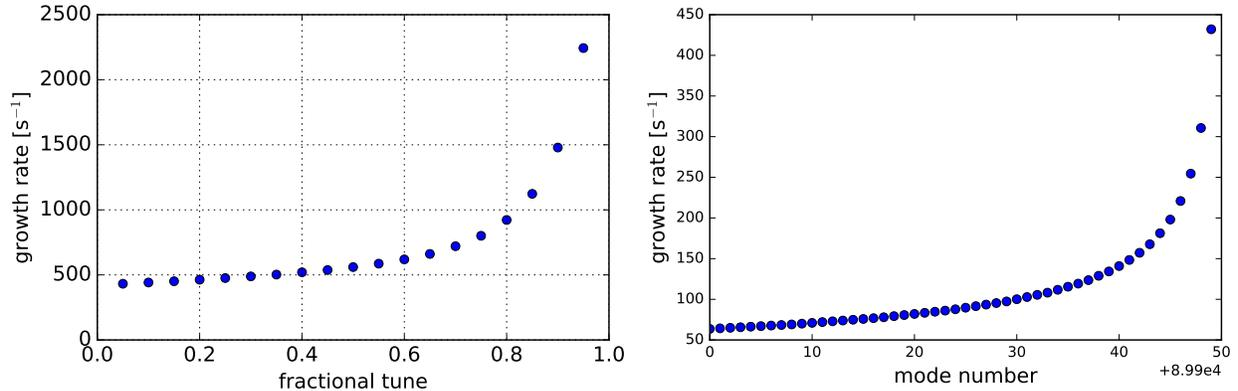
FIG. 12. Growth rate as a function of the fractional tune for the most dangerous coupled bunch mode (left), and as a function of the coupled bunch mode number for the case with  $\nu_\beta = 0.05$  (right).
