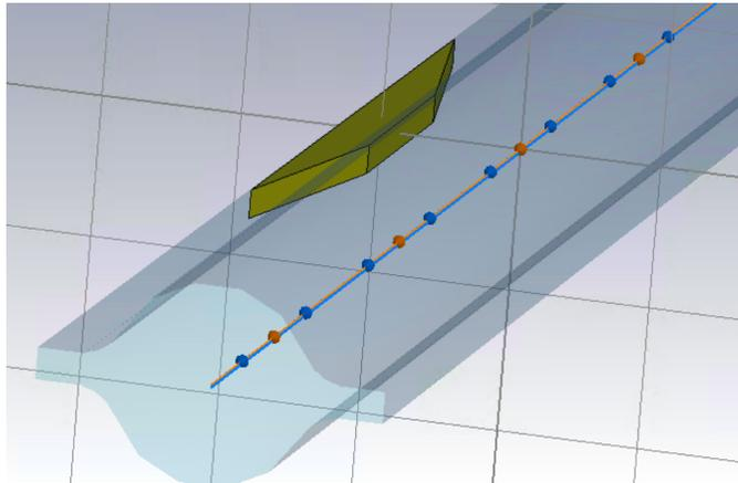
FIG. 16. 3D model of the FCC-ee vacuum chamber with winglets and a synchrotron radiation absorber used for CST simulations.
