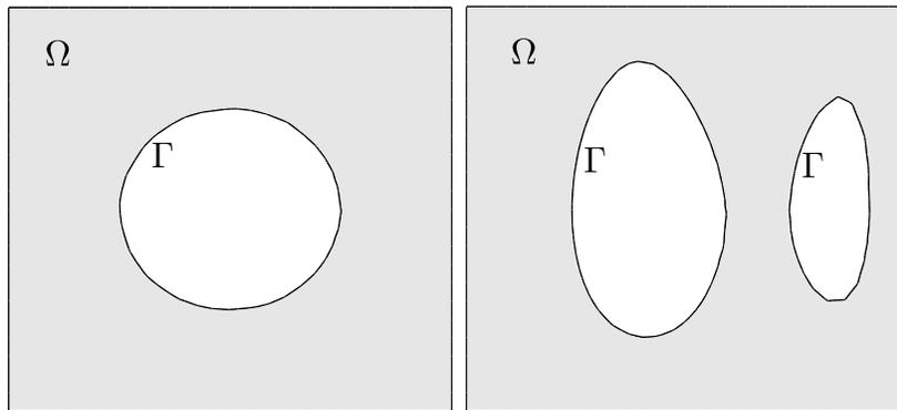
Figure 1: The final domain (left) and initial guess (right) for Model Problem 1. The gray area is the computational domain  $\Omega$ , the outer square boundary is fixed, and  $\Gamma$  is the free boundary.
