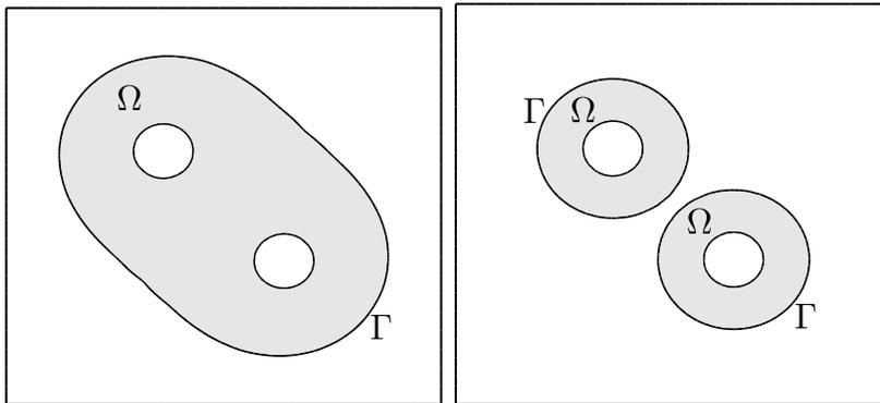
Figure 2: The final domain (left) and initial guess (right) for Model Problem 2. The gray area is the computational domain  $\Omega$ , the outer square boundary and the two inner most circles are fixed, and  $\Gamma$  is the free boundary.
