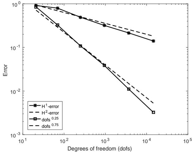
Figure 3: Convergence of the error in velocity field in Model Problem 1 in the  $H^1$  and  $L^2$ -norm.
