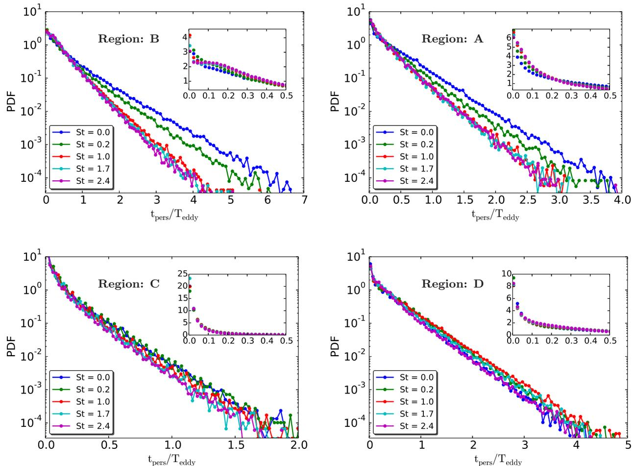
FIG. 4: (Color online) Semi-log plots of the persistence-time PDFs  $P_\phi(t_{\text{pers}})$  of the times  $t_{\text{pers}}$  for the four regimes in the  $Q - R$  plane, for different Stokes numbers; the inset shows  $P_\phi(t_{\text{pers}})$  for small  $t_{\text{pers}}$ .
