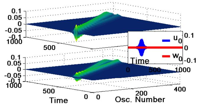
FIG. 4: The two soliton regime: Combining solutions corresponding to two different modes(lower dashed line in [Fig.3]), we generate a soliton wave through the upper chain, while the lower chain is being at rest. As a result due to different velocities solitons depart from each other and propagate independently through the system. Corresponding frequency and amplitude:  $\Omega = 1.90$ ,  $A = 0.025$
