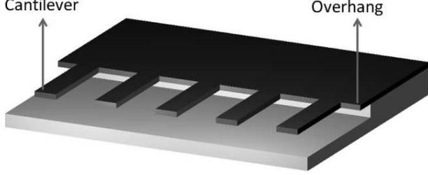
FIG. 2: The scheme of a mono-element cantilever array. Exactly same cantilevers are linked by means of the overhang, thus any particular cantilever can be represented as an oscillator.
