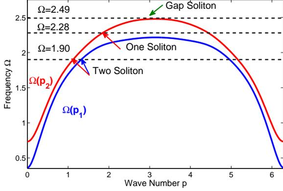
FIG. 3: The dispersion relation for the considered system of two weakly coupled cantilever arrays. The blue and red curves represent dispersion relations for  $p_1$  and  $p_2$  respectively. As a result of these relations we consider three regimes: a) Two Soliton (lower dashed line), b) One soliton (middle dashed line), c) Amplification scenario (upper dashed line), with respective frequencies.
