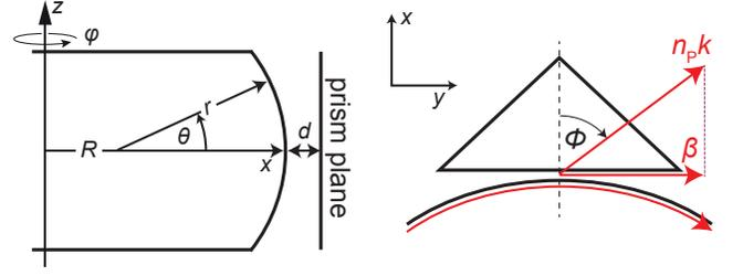
FIG. 1. (Left) Coordinate system and geometrical parameters considered in this work. (Right) Illustration of the coupling condition within the ray optics picture.
