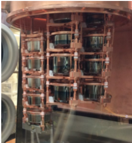
Figure 2: Module 2 detectors being installed.
