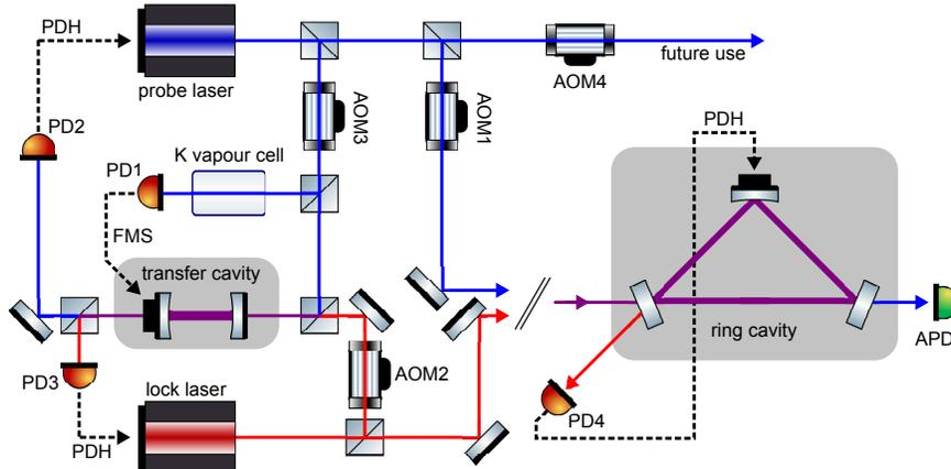
FIG. 2. Simplified schematic of the cavity lock and probe laser systems. The lock laser operates at 852 nm and the probe laser at 770 nm. AOM: acousto-optic modulator; PD: photodiode; APD: avalanche photodiode; FMS: frequency modulation spectroscopy; PDH: Pound-Drever-Hall. All AOMs are in double-pass configuration. AOM1 tunes the probe beam, whose transmitted power is detected at the APD, AOM2 tunes the ring cavity, and AOM3/AOM4 are reserved for future experiments.
