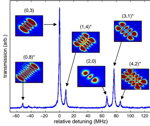
FIG. 3. Transverse cavity modes. The solid curve shows a number of cavity transmission resonances (without atoms), and insets show the corresponding spatial profiles as imaged onto a camera. The 45° tilt of the patterns reflects the orientation of the cavity plane ( $\hat{\kappa}_\perp$ ). The modes are labelled according to transverse indices  $(m, n)$ , with asterisks denoting a longitudinal index  $q$  which is one less than that of the  $(0, 3)$  mode which is taken as reference.
