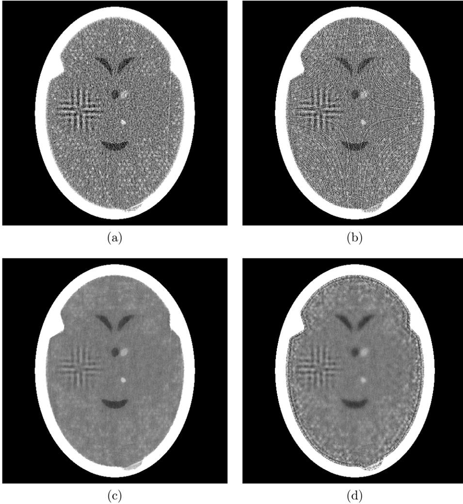
Figure 4: Reconstructions from 720 projections by (a) filtered back-projection, (b) the algorithm ART, (c) TV-Based Superiorized Version of ART, and (d) Shearlet-Based Superiorized Version of ART.
