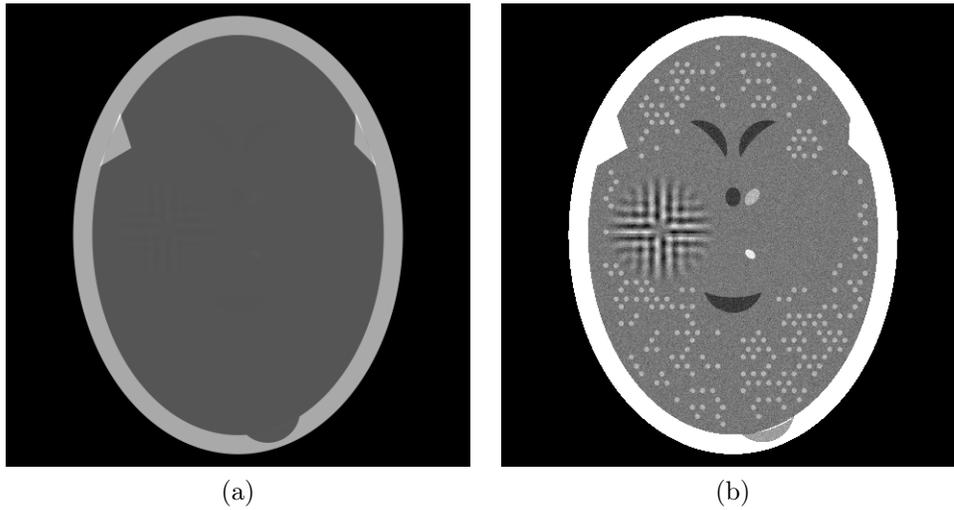
Figure 1: A  $485 \times 485$  digitization of a phantom based on the distribution of x-ray attenuation in units of  $\text{cm}^{-1}$  within a transaxial slice of the human head. We display in (a) 0.000 as black and any value that is 0.6241749 or greater as white, in (b) 0.20400 as black and any value that is 0.21675 or greater as white. The latter mapping of values into displayed intensities is used for all the images shown below.
