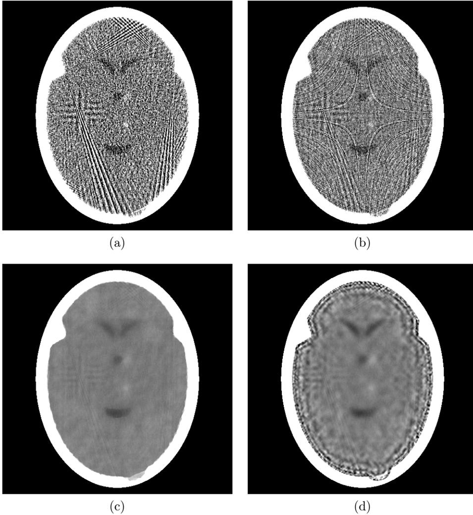
Figure 2: Reconstructions from 180 projections by (a) filtered back-projection, (b) the algorithm ART, (c) TV-Based Superiorized Version of ART, and (d) Shearlet-Based Superiorized Version of ART.
