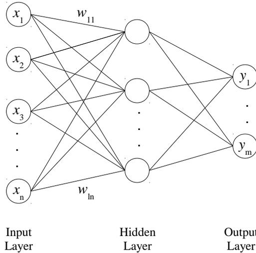
**Fig. 6: A Multi Layered Feed-Forward Network**
