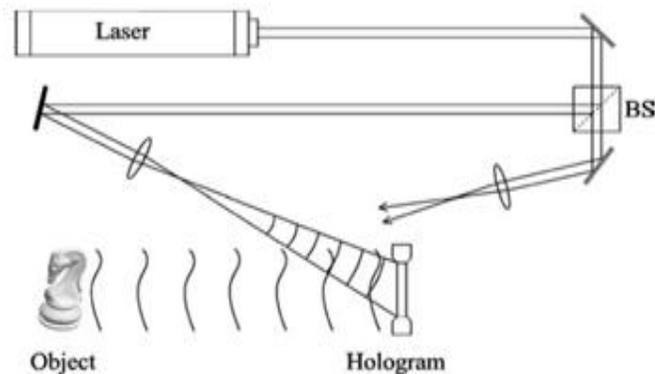
**Fig. 1: Hologram Recording**
