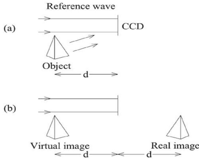
**Fig.3: Digital holography: (a) recording, (b) reconstruction.**
