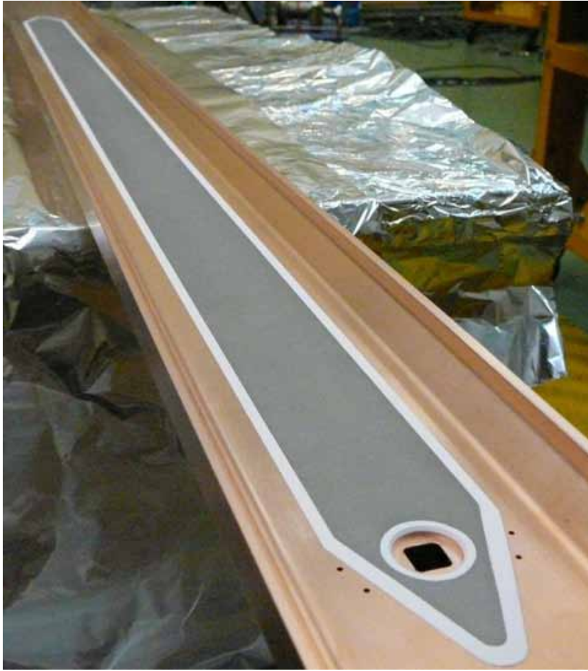
Figure 23. Photo of deposited electrode on the bottom of the SCW beam pipe.
