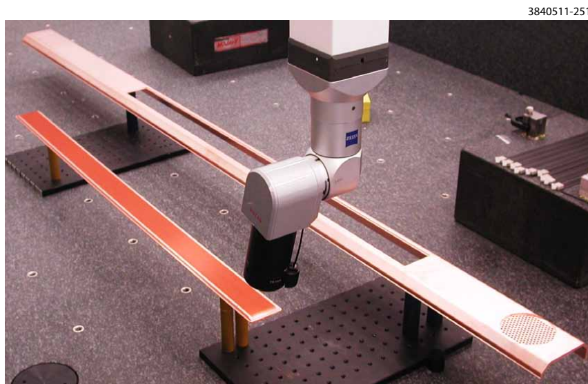
Figure 16. Bottom half of an SCW beam pipe with a cut-out and the groove plate during inspection on a CMM (Photo courtesy of Dawn Munson of LBNL)
