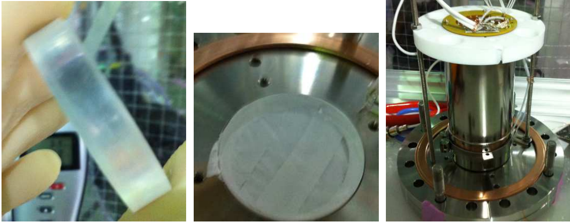
Figure 2. Left: undoped cylindrical CsI crystal with its side surfaces roughly polished. Middle: the crystal embedded into the customized Conflat flange with its bottom and side surfaces wrapped with Teflon tape. Right: PMT mounted on top of the crystal with its photo-cathode facing downward.
