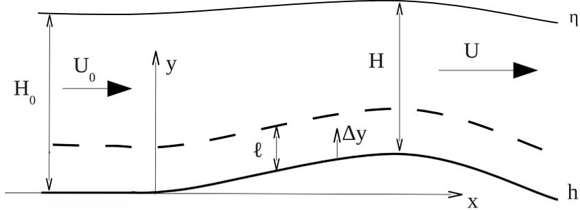
Figure 1: Definition of the free surface  $\eta$ , the bedform height  $h$ , the liquid depth  $H$ , the fluid velocity  $U$  in the outer region, the height of the inner region  $\ell$ , the vertical coordinate employed in the outer region  $y$  and the displaced vertical coordinate employed in the inner region  $\Delta y$ . The subscript 0 corresponds to the fluid flow over a flat bed.
