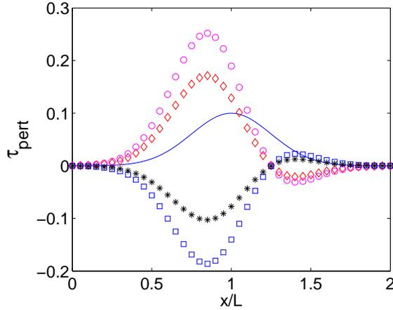
Figure 2: Longitudinal evolution of the perturbation of the shear stress  $\tau_{pert}$ , for different Froude Numbers  $Fr$ . The symbols  $\diamond$ ,  $\circ$ ,  $\square$  and  $*$  correspond to  $Fr = 0.5$ ,  $Fr = 0.7$ ,  $Fr = 1.3$  and  $Fr = 1.5$ , respectively. The continuous line corresponds to the normalized bedform  $h/H_0$ .
