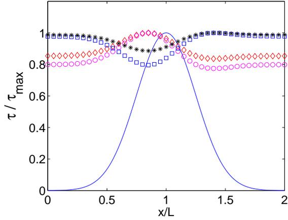
Figure 3: Longitudinal evolution of the normalized shear stress  $\tau/\tau_{max}$ , for different Froude Numbers  $Fr$ , where  $\tau_{max}$  is the maximum of the shear stress. The symbols  $\diamond$ ,  $\circ$ ,  $\square$  and  $*$  correspond to  $Fr = 0.5$ ,  $Fr = 0.7$ ,  $Fr = 1.3$  and  $Fr = 1.5$ , respectively. The continuous line corresponds to a normalized bedform  $h/h_{max}$ , where  $h_{max}$  is the maximum height of the bedform.
