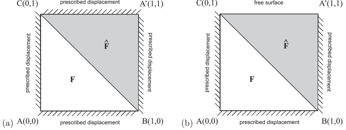
Figure 3: Elastic square with (a) Dirichlet boundary conditions and (b) with one side left free and Dirichlet boundary conditions on the other three sides, partitioned into two right-angled triangles with homogeneous deformation gradient in each triangle.
