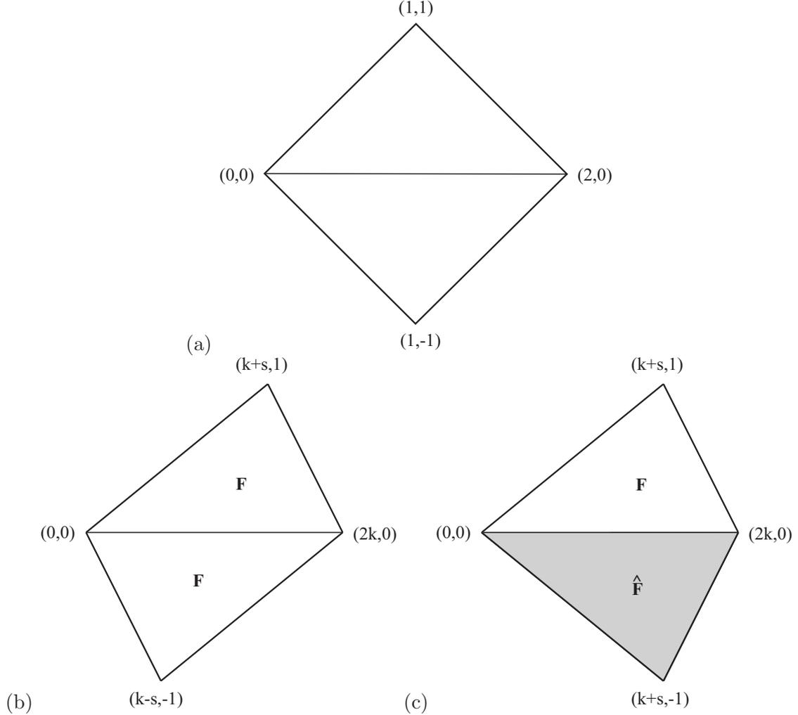
Figure 7: Elastic square partitioned into two right-angled triangles, showing: (a) the reference configuration, (b) the deformed state with the deformation gradient equal to  $\mathbf{F}$  on each triangle, (c) the deformed state with the deformation gradient equal to  $\mathbf{F}$  on one triangle and  $\widehat{\mathbf{F}}$  on the other.
