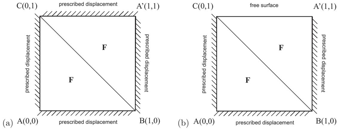
Figure 5: Elastic square with (a) uniform Dirichlet boundary conditions and (b) with one free side and Dirichlet boundary conditions on the remaining three sides, partitioned as two right-angled triangles, and the corresponding homogeneous deformation gradient indicated in each triangle.
