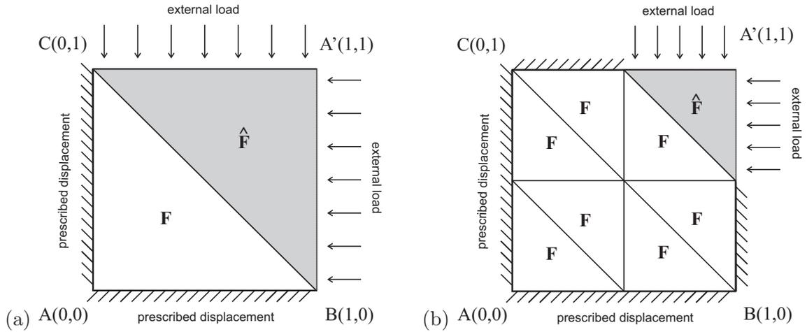
Figure 4: Elastic square with mixed boundary conditions, partitioned into right-angled triangles with homogeneous deformation gradient in each triangle.
