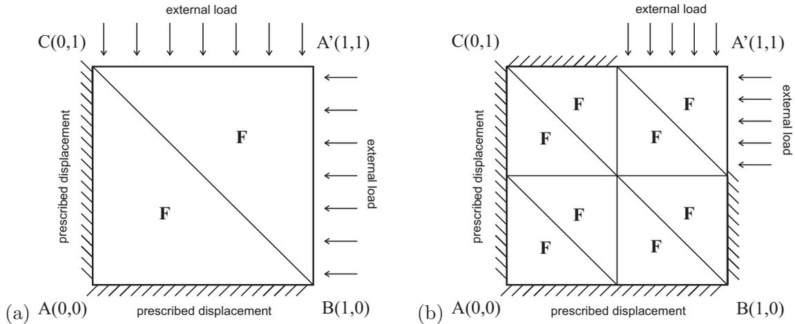
Figure 6: Elastic square with mixed boundary conditions, partitioned as two right-angled triangles, and the corresponding homogeneous deformation gradient indicated in each triangle.
