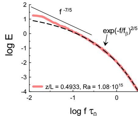
FIG. 2: Temperature spectrum measured at  $Ra = 1.08 \times 10^{15}$  and Prandtl number  $Pr = 0.8$  near the horizontal midplane. The dashed line indicates the spectral law Eq. (5) with  $\beta = 2/5$ .
