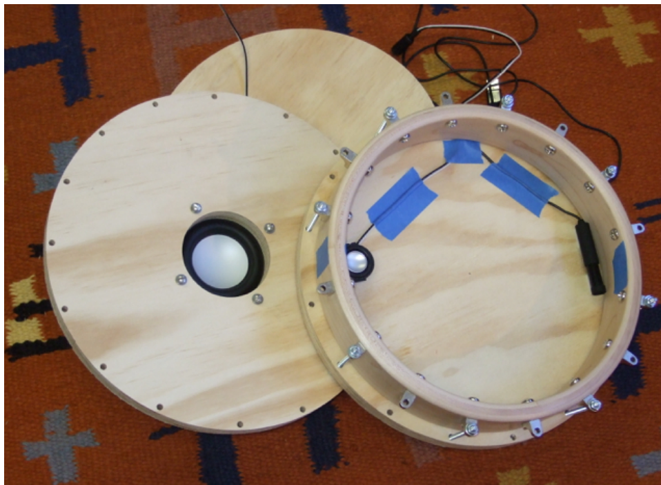
FIG. 3. Speaker and microphone mounted internally on a solid plywood head and a second plywood disk to close the back; also the head-speaker combination used for FIG.s 6 and 9
