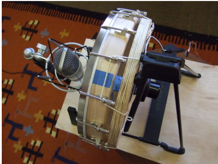
FIG. 8. Set-up for one of the traces in FIG. 9: shallow pot; plywood/speaker back, angled with a 3/8'' spacer; mic 2'' from the center of the head
