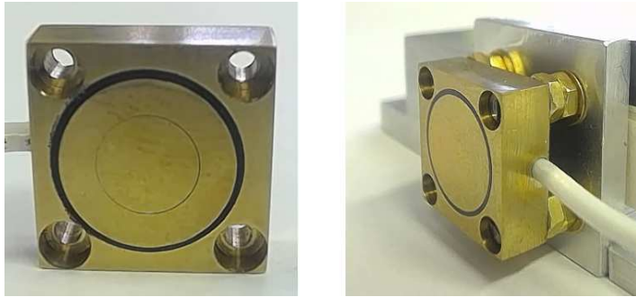
Figure 4. The brass electrodes forming the capacitive distance sensor. The probe and guard electrodes are circular and concentric, and fit into a square outer frame with screw holes for mounting.
