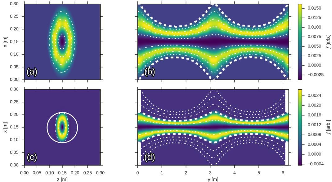
FIG. 8: Heat map of  $f$  in diffusion model at  $t = 400$ . (a): no limiter, (b): circular limiter. Solid black lines indicate size and position of limiter. Dashed black lines indicate position of last closed flux surface. Dot-dashed lines show positions of flux surfaces. Note that these figures have been upscaled in post-processing following the procedure outlined in section VB.
