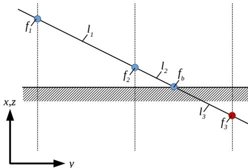
FIG. 2: A field line leaving the boundary.  $f_2$  is located on a grid point, while  $f_1, f_3$  are located on intersection points with the adjacent perpendicular planes, and  $f_b$  is located on the intersection with the boundary.  $l_1, l_2, l_3$  are distances along the field lines between the four points above.
