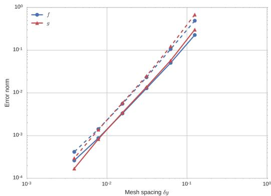
FIG. 4: Error scaling for the 3<sup>rd</sup>-order LVF scheme in BOUT++. Solid lines are the  $l_2$  norm, dashed lines are the  $l_\infty$  norm (i.e. max. error).
