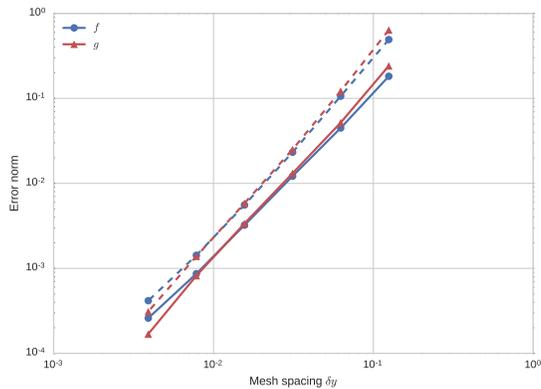
FIG. 3: Error scaling for the 2<sup>nd</sup>-order LVF scheme in BOUT++. Solid lines are the  $l_2$  norm, dashed lines are the  $l_\infty$  norm (i.e. max. error).
