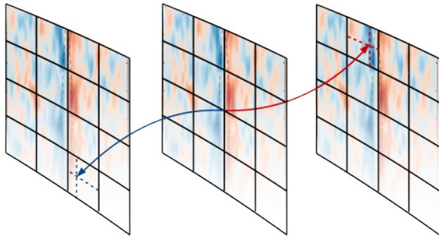
FIG. 1: Schematic of the Flux Coordinate Independent method for the parallel derivative operator. Starting from a given grid point, magnetic field lines are traced in the forward and backward directions. The argument of the operator is interpolated to find the value at the location where the field line intersects the adjacent perpendicular slices, allowing a finite difference scheme to be constructed.
