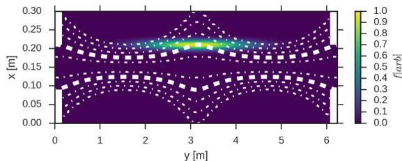
FIG. 7: Heat map of initial condition for  $f$  in diffusion model in the  $(x, y)$  plane at  $z = 0.15$ . Solid black lines indicate size and position of limiter. Dashed black lines indicate position of last closed flux surface. Dot-dashed lines show positions of flux surfaces.
