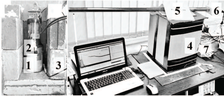
Figure 1: On left: NaI spectrometer inside lead shield (front side of shield removed). 1) \phi 63 \times 63 mm NaI(Tl) scintillator, 2) R6091 PMT, 3) lead bricks. On right: NaI and ^3\text{He} neutron spectrometers during data acquisition. 4) Black box with NaI detector inside, 5) CHM-57 ^3\text{He} filled proportional counter, 6) ^3\text{He} neutron detector's preamplifier, 7) DT5780 Dual Digital Multi Channel Analyzer used to acquire data from both detectors.
