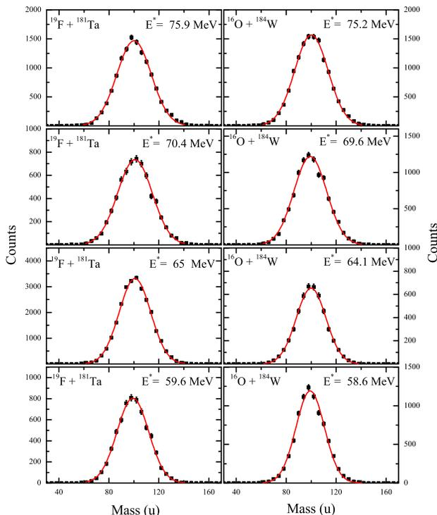
FIG. 2. (Color online) Experimental mass distributions of fission fragments for the reactions  $^{19}\text{F} + ^{181}\text{Ta}$  (left) and  $^{16}\text{O} + ^{184}\text{W}$  (right) at different excitation energies. They were fitted by single Gaussian shown by full (red) lines.
