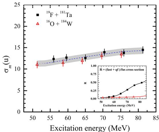
FIG. 3. (Color online) Variation of the standard deviation  $\sigma_m(u)$  of the fitted symmetric mass distribution with excitation energy. The calculated widths are shown in (blue) dashed line, the shaded region indicate uncertainties in calculation (see text). The predicted [8] variation of the sum of the fast fission and quasi-fission cross sections (normalized with respect to the fusion cross sections) with excitation energy are presented in the inset.
