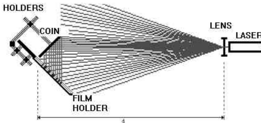
**Figure 3: Holographic setup**
