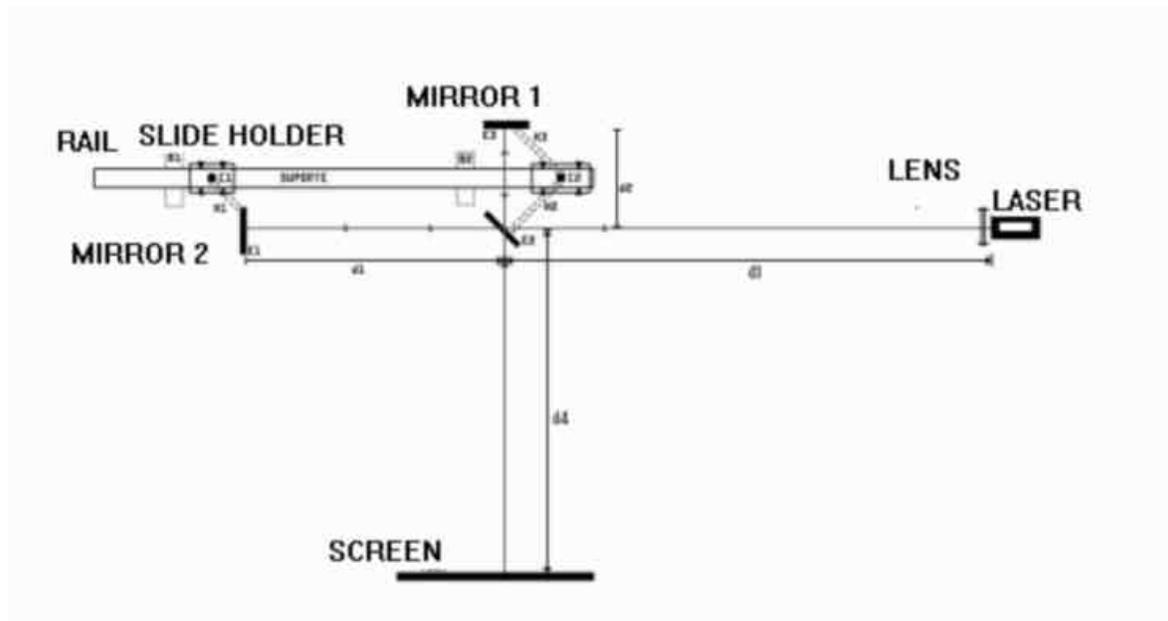
**Figure 1: Michelson interferometer setup**
