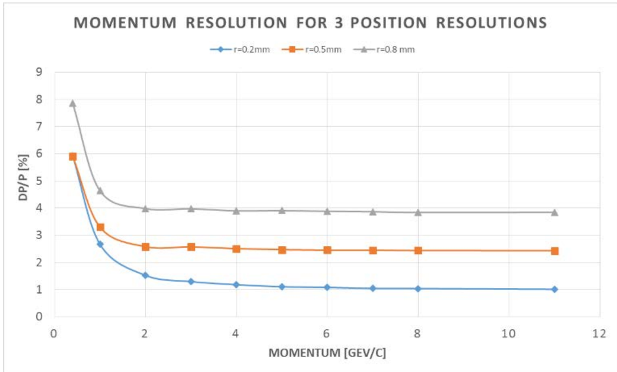
Figure 23: Momentum resolution of the spectrometer for three different position resolutions, namely 0.2, 0.5 and 0.8 mm
