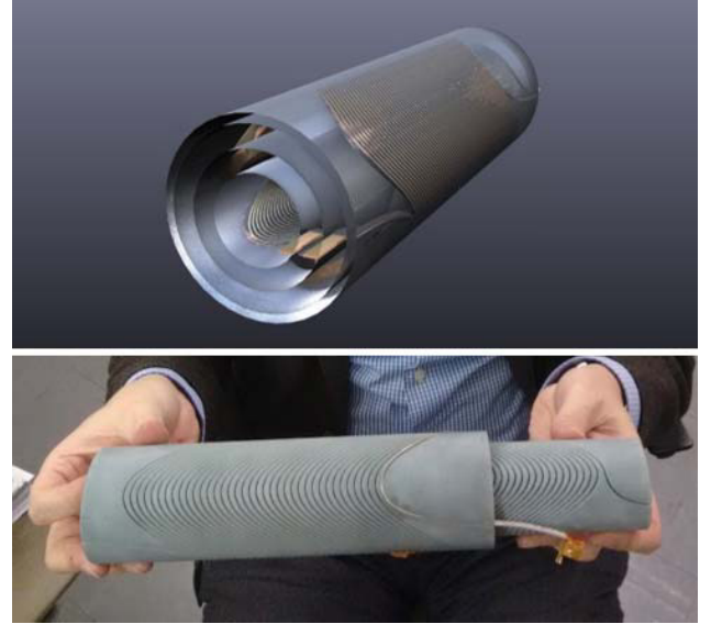
Figure 3: Prototype CCT final focus quadrupole. CAD drawing (top) and 3D printed item (bot).
