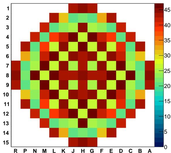
Fig. 3. An example of the reactor core map of fuel elements with different burn-up (unit:  $\text{GW} \cdot \text{day} \cdot \text{ton}^{-1}$ ) shown in color scale at the end of a refueling cycle.
