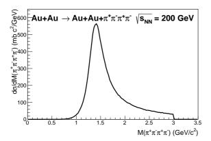
Figure 5: Parent mass distribution for 4-pion final state produced in Au+Au collisions at RHIC energies. The 3  $\text{GeV/c}^2$  cutoff is due to the choice of  $W_{\text{MAX}}$ .
