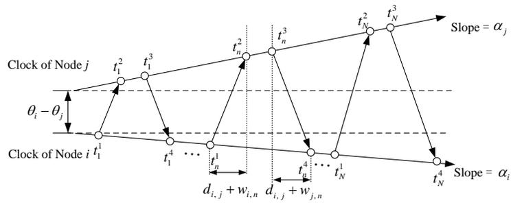
Fig. 2. Two way message exchange between node  $i$  and  $j$  in the WSN.
