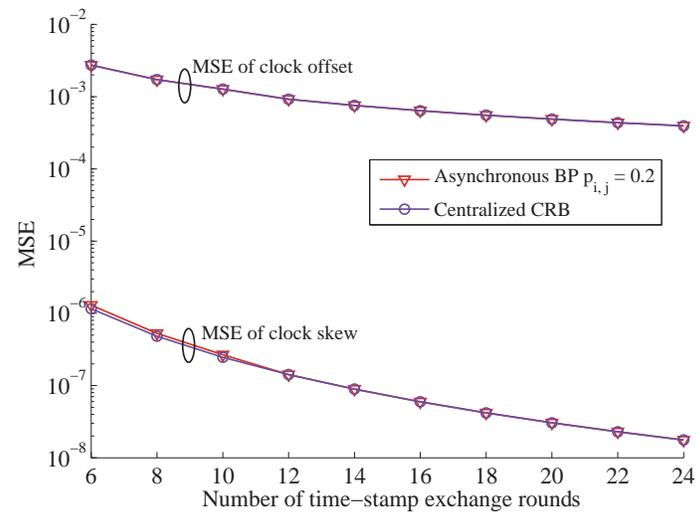
Fig. 6. MSE of clock skew and offset averaged over the whole network under random network topologies.
