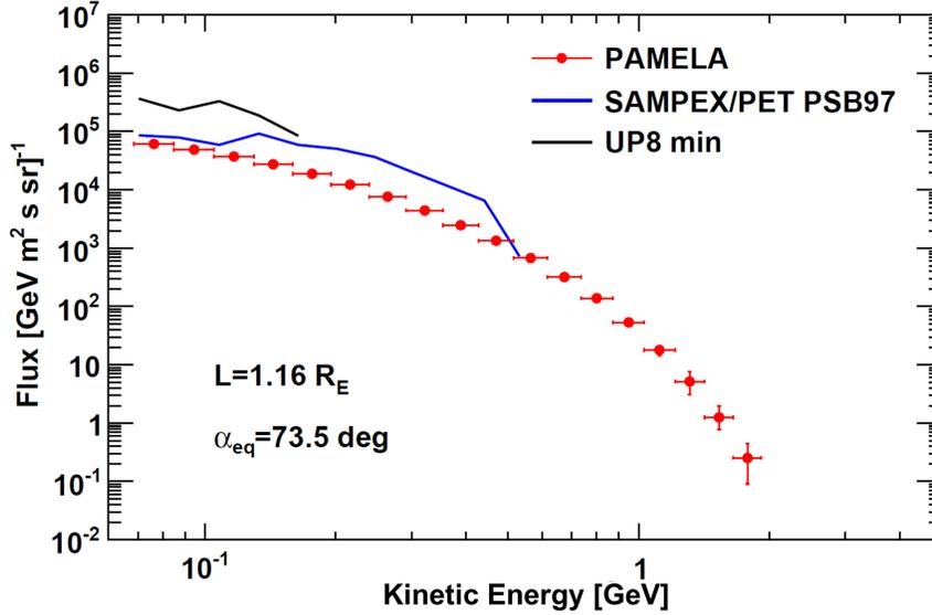
Fig. 1.— PAMELA trapped proton energy spectrum for sample  $\alpha_{eq}$  and  $L$ -shell values, compared with the predictions from the UP8-min (Sawyer & Vette 1976) and the PSB97 (Heynderickx et al. 1999) models (from SPENVIS, <https://www.spennis.oma.be/>).
