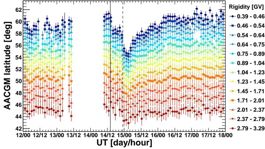
Fig. 6.— Time profile of the geomagnetic cutoff latitudes measured by PAMELA, for different rigidity bins. Vertical solid and dashed lines mark the shock and the magnetic cloud arrival, respectively.
