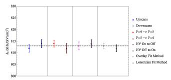
FIG. 9. Data subset comparisons to investigate potential systematic errors. The comparisons are between: scan direction, intermediate hyperfine transition, HV switching direction, and Stark shift fitting/ extraction method.
