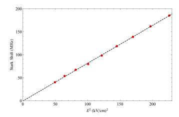
FIG. 7. Magnitude of measured shift vs. the square of the applied electric field. The result of one day's worth of data is shown, with all runs taken at a given electric field value averaged. Statistical errors of each point are comparable to the point size. The Stark shift constant  $|k_S|$  (slope of fitted line) has an uncertainty of about 1% for these data.
