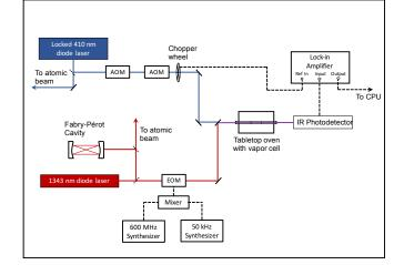
FIG. 3. A schematic diagram detailing the supplementary indium vapor cell used for obtaining the hyperfine peaks as a reference signal and RF sidebands for frequency calibration.
