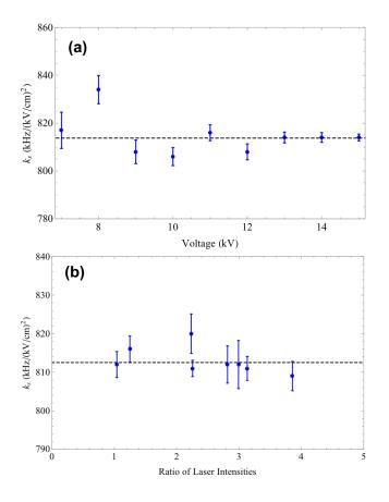
FIG. 10. (a) Correlation plot of  $|k_S|$  vs. electric field. No statistically resolved slope is observed. (b) Correlation plot of  $|k_S|$  vs. the ratio of blue to IR laser intensities. No statistically resolved slope is observed.
