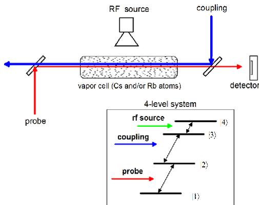
FIG. 1. Illustration of a four-level system, and the vapor cell setup for measuring EIT, with counter-propagating probe and coupling beams. The RF is applied transverse to the optical beam propagation in the vapor cell.
