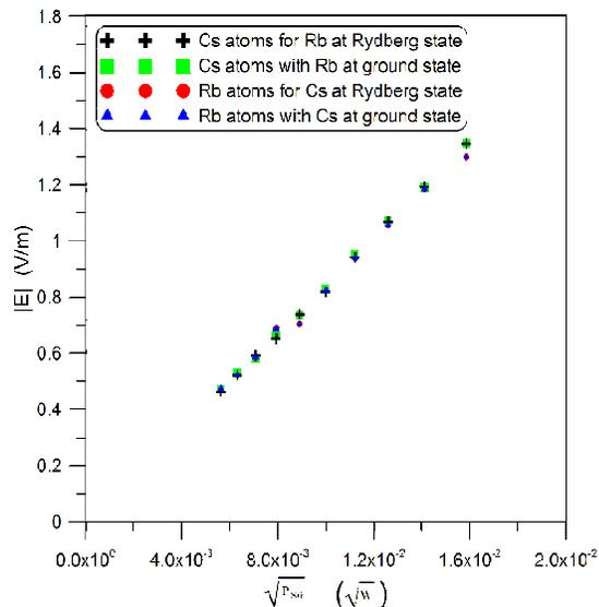
FIG. 11. Calculated  $|E|$ -field as a function of SG power for the  $^{133}\text{Cs}$  at  $f_{RF}=13.4016$  GHz and  $^{85}\text{Rb}$  at  $f_{RF}=13.4375$  GHz. Comparison of measured  $|E|$ -field with both atoms at Rydberg states and for one atom at ground state where no significant systematic atom-atom effects are observed.
