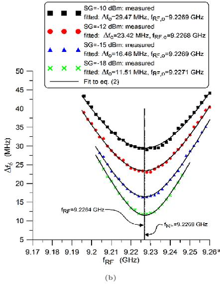
FIG. 5. RF detuning experiments: (a)  $^{133}\text{Cs}$ :  $43D_{5/2}-44P_{3/2}$  and (b)  $^{85}\text{Rb}$ :  $61D_{5/2}-62P_{3/2}$ . The vertical lines and corresponding frequencies are the  $f_{RF,o}$  obtained from both the RF detuning measurements and from the quantum defect data.
