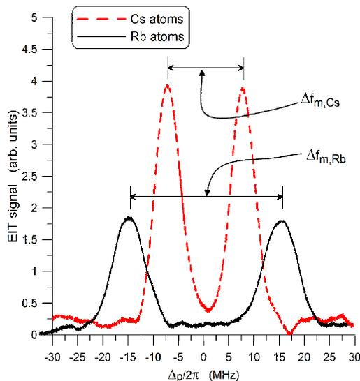
FIG. 4. Illustration of the EIT signal (i.e., probe laser transmissions through the cell) as a function of probe laser detuning  $\Delta_p$ . The dashed line is the measured EIT signal obtained with the Cs atoms and the solid line is the measured EIT signal obtained with the Rb atoms. The observed splitting result from an applied 9.222 GHz RF  $E$ -field.
