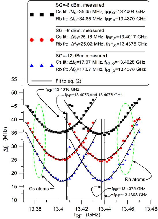
FIG. 9. RF detuning experiments for both  $^{133}\text{Cs}$  ( $66S_{1/2}$ - $66P_{3/2}$ ) and  $^{85}\text{Rb}$  ( $65S_{1/2}$ - $65P_{3/2}$ ). The vertical lines and corresponding frequencies are the  $f_{RF,o}$  obtained from both the RF detuning measurements and from the quantum defects.
