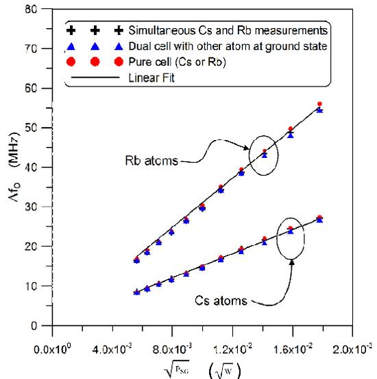
FIG. 8. Comparison of measured  $\Delta f_o$  with dual cell (with both atoms at Rydberg state or for one atom at ground state) and for a pure cell:  $^{133}\text{Cs}$  at  $f_{RF}=9.218$  GHz and  $^{85}\text{Rb}$  at  $f_{RF}=9.227$  GHz.
