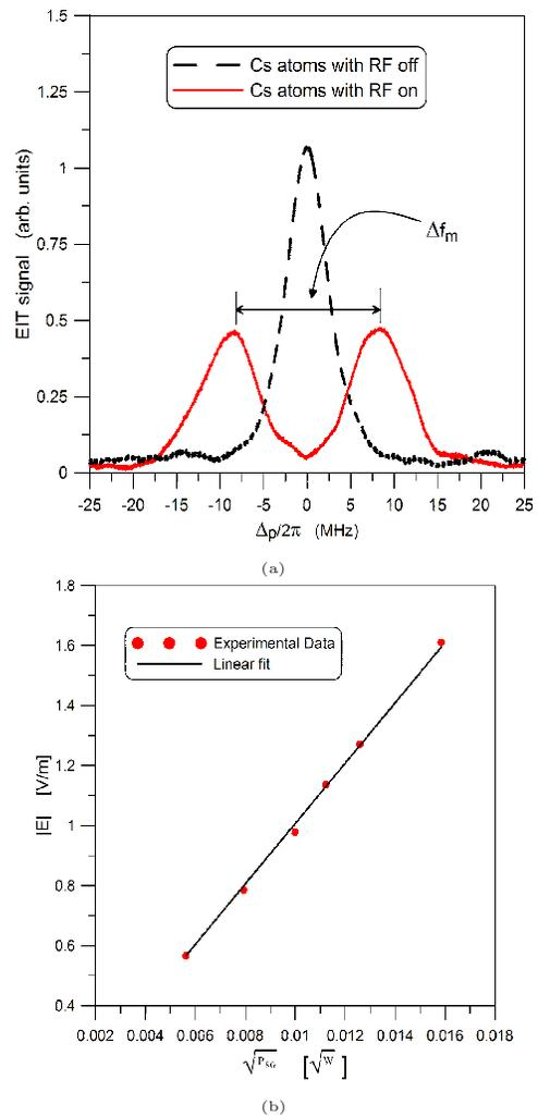
FIG. 2. This dataset is for an RF of 13.404 GHz and corresponds to the following 4-level Cs atomic system:  $6S_{1/2} - 6P_{3/2} - 66D_{5/2} - 66P_{3/2}$ . (a) Illustration of the EIT signal (i.e., probe laser transmission through the cell) as a function of probe laser detuning  $\Delta p$ . (b) Calculated E-field for a given signal generator power  $P_{SG}$ , see discussion below.
