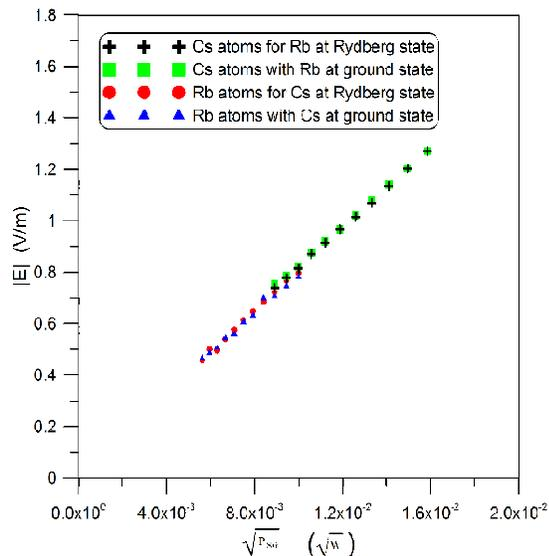
FIG. 13. Calculated  $|E|$ -field as a function of SG power for the  $^{133}\text{Cs}$  at  $f_{RF}=11.6172$  GHz and  $^{85}\text{Rb}$  at  $f_{RF}=11.6656$  GHz. Comparison of measured  $|E|$ -field with both atoms at Rydberg states and for one atom at ground state where no significant systematic atom-atom effects are observed.
