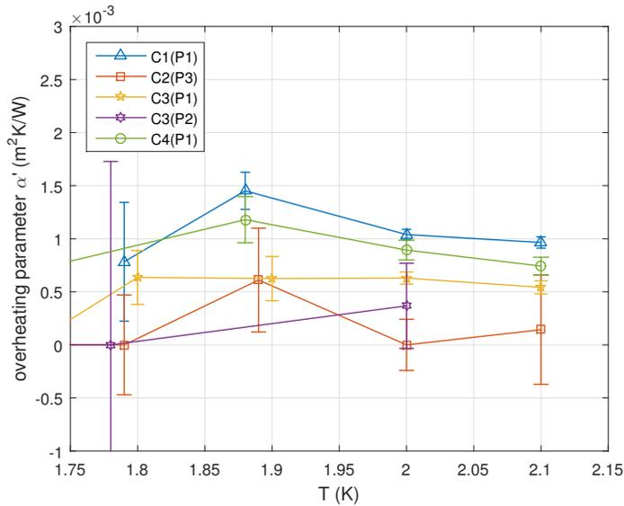
(c) Normalized overheating parameter  $\alpha'$  plotted over temperature for many cavities.
