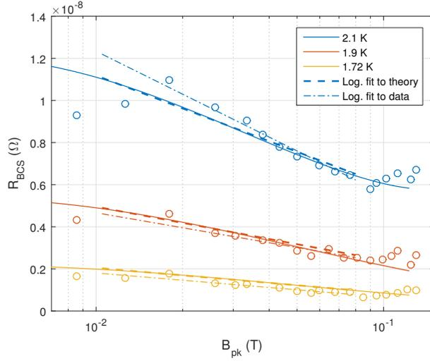
Figure 5: C3(P1) results with logarithmic fitting to both experimental data and theoretical predictions. Both show approximate logarithmic behavior in the medium-field region. The plot has been limited to three temperatures to reduce visual clutter.
