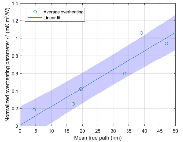
(d) Average normalized overheating parameter  $\alpha'$  plotted as a function of mean free path, with a linear fit. Shaded region indicates  $1\sigma$  confidence interval.
