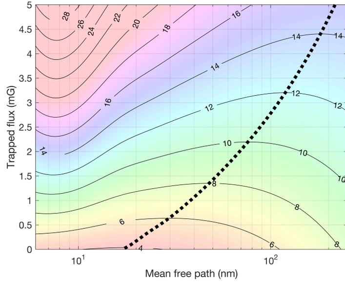
Figure 7: Total surface resistance  $R_s = R_{\text{BCS}}(\ell, 2 \text{ K}, 16 \text{ MV/m}) + R_0(\ell, B_{\text{trapped}})$  over mean free path and trapped flux. Contour labels are given in  $\text{n}\Omega$ . Heavy dashed line indicates optimal mean free path for a given amount of trapped flux.
