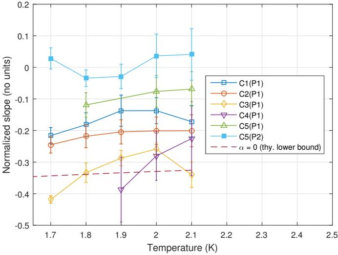
(a) Normalized logarithmic slopes of the surface resistance in field, as defined in Eq. 7, plotted over temperature. Dashed line indicates the theoretical normalized slope for zero overheating.
