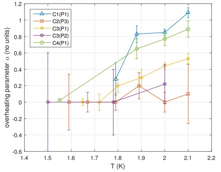
(b) Overheating parameter  $\alpha$  plotted over temperature for many cavities.
