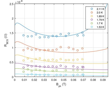
(c) Test of cavity C5(P1), with  $\ell = 60 \pm 18$  nm,  $\alpha(2.11 \text{ K}) = 1.7$ .
