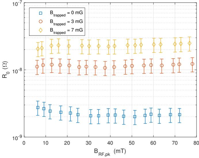
(a) Representative  $R_0$  vs.  $B_{\text{RF,pk}}$  for a 1.3 GHz TESLA cavity, at varying levels of trapped magnetic flux.
