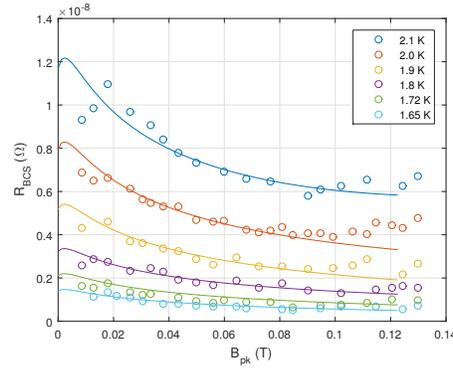
(b) Test of cavity C3(P1), with  $\ell = 34 \pm 10$  nm,  $\alpha(2.1 \text{ K}) = 0.44$ .
