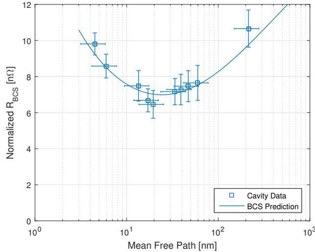
Figure 2: At low field ( $\sim 5$  MV/m), the measured BCS resistance (normalized to an average energy gap  $\Delta$  and critical temperature  $T_c$ ) at 1.3 GHz and 2 K, plotted as a function of electron mean free path, shows an agreement with the theoretical minimum of  $25 \pm 1$  nm.
