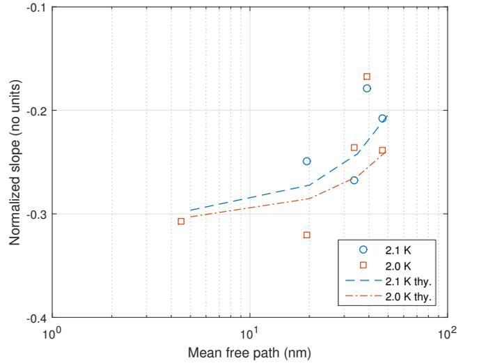
(b) Normalized logarithmic slopes of the surface resistance in field, plotted over mean free path. The plot has been limited to two temperatures to reduce visual clutter.
