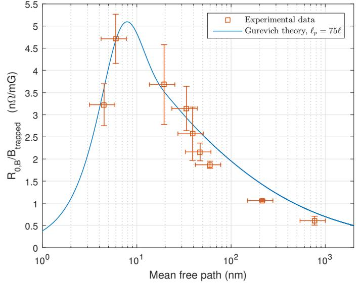
(b) Experimental data and theoretical prediction for sensitivity of residual resistance to trapped magnetic flux as a function of mean free path.
