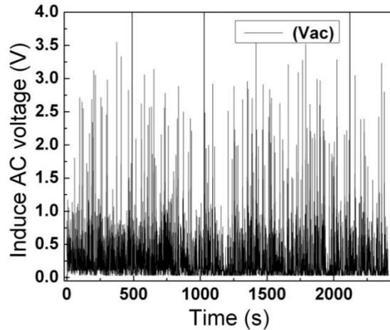
**Figure 5:** Graph of induced AC voltage in the coil with respect to time.
