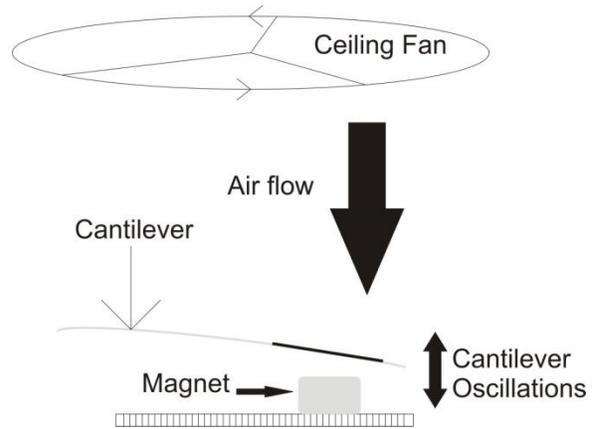
**Figure 2:** Schematic shows the side view of the testing of the harvester arranged under the ceiling fans. Only one fan is shown. Distance between the fan and the surface of the cantilever was measured to be 2.66m.
