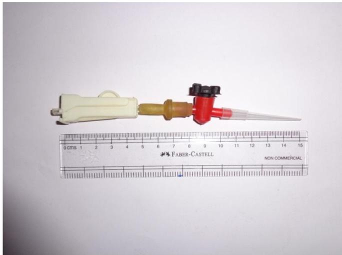
The dispenser was characterized by depositing a droplet from the dispenser nozzle on to the microbalance under the action of gravity and its mass was measured. Using the equation (I) and from the values of the density of water and its measured mass, the diameter of the droplet was calculated. Table – 1 below shows the values for the characterization of water droplet.
