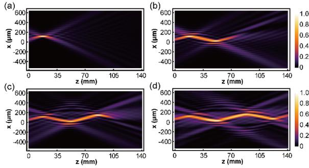
Fig. S2. The intensity distribution of the 1D sine beams with increasing number of segments in the superposition process. The 1D sine beam with two periods is selected to demonstrate in the main text, but it is worth noting that more bends are available in principle.
