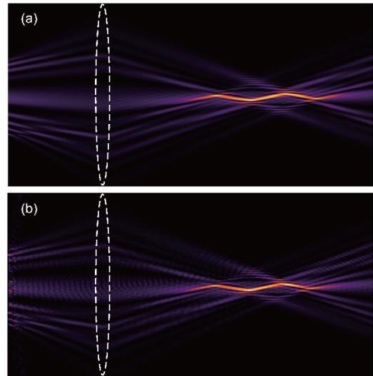
Fig. S1. The influence of the quasi-grey-scale amplitude modulation on the pre-designed 1D sine beam. The amplitude distribution for the propagation of 1D sine beam under (a) ideal and (b) quasi-grey-scale amplitude modulation, where the dashed line indicates the position of the lens. The amplitude rather than the intensity distribution is presented to highlight the area with weak optical intensity.
