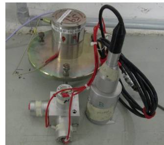
Figure 3: HLS, tri-axial geophone and seismometer.
