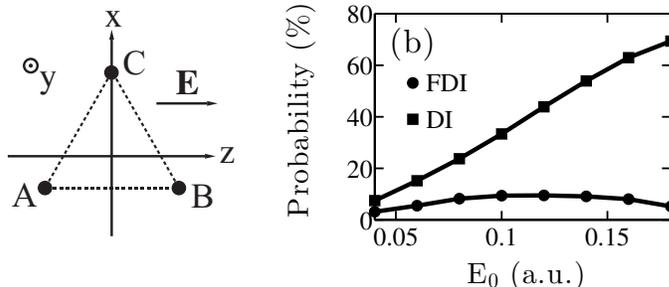
**Figure 4.** Left panel: The initial configuration of the nuclei in the  $H_3^+$  triatomic molecule. The laser pulse is linearly polarized and aligned along one side of the triatomic molecule. Right panel: The DI and FDI probabilities as a function of the laser field strength  $E_0$ . The lowest laser field strength in (b) is  $E_0 = 0.04$  a.u..
