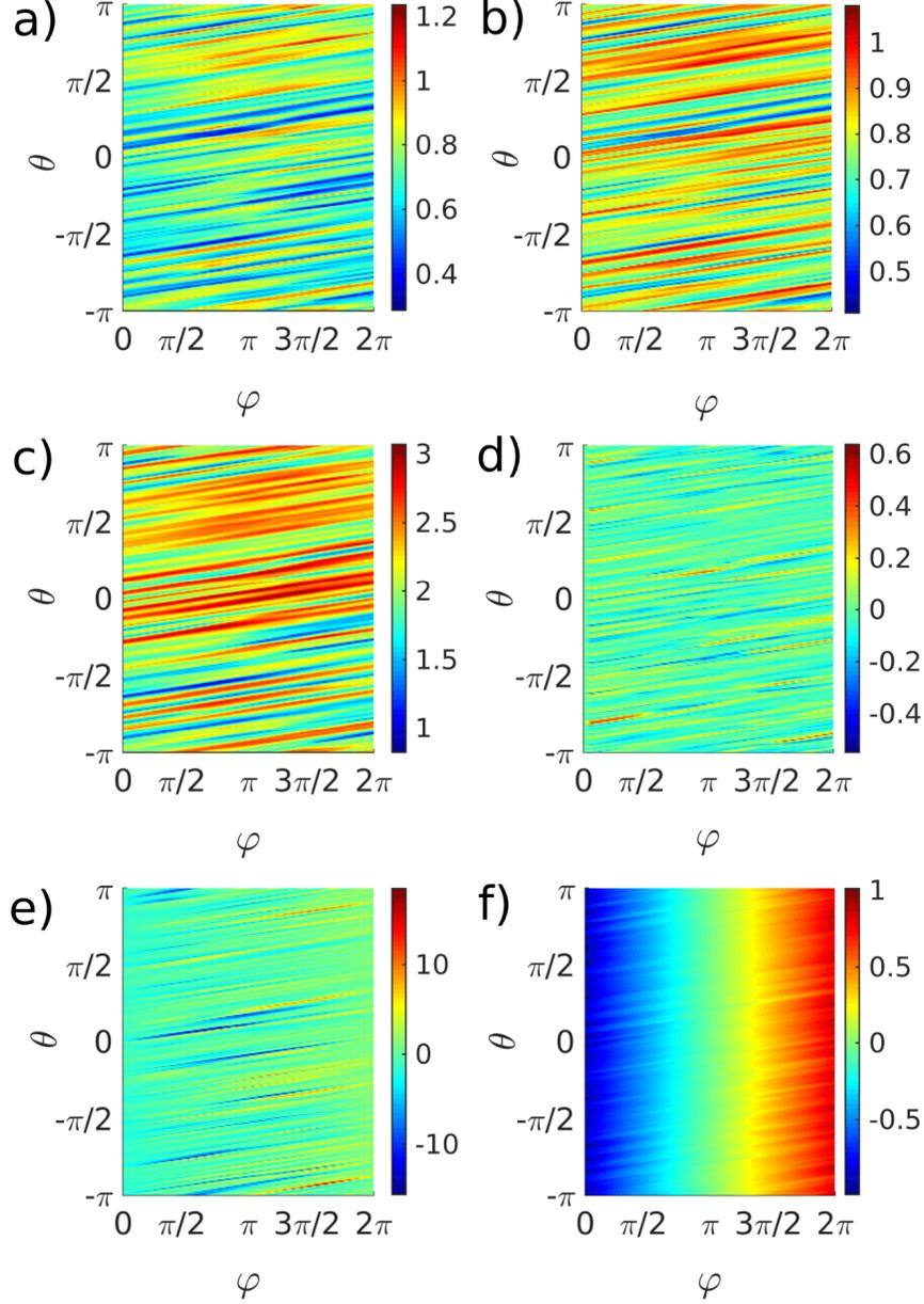
FIG. 2. Snapshots of plasma turbulence for the standard ISTTOK simulation on a toroidal cross section at  $x = x_s + 5 \rho_{s0}$ . We show: (a) plasma density  $n/n_0$ , (b) electron temperature  $T_e/T_{e0}$ , (c) electrostatic potential  $\phi/eT_{e0}$ , (d) vorticity  $\omega = \rho_{s0}^2 \nabla_{\perp}^2 \phi/eT_{e0}$ , (e) electron  $V_{\parallel e}/c_{s0}$ , and (f) ion  $V_{\parallel i}/c_{s0}$  parallel velocities.
