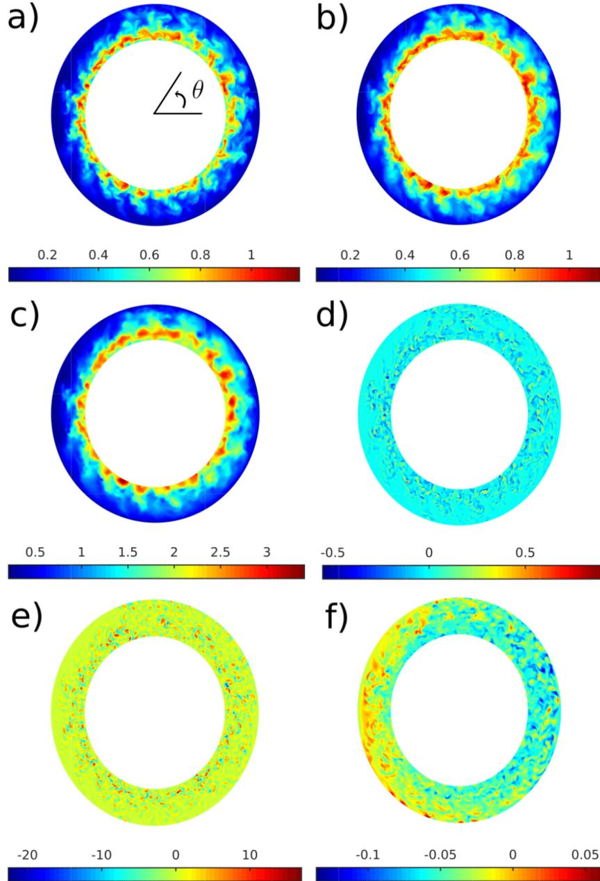
FIG. 1. Snapshots of plasma turbulence in the standard ISTTOK simulation on a poloidal cross section halfway between the limiter plate ( $\varphi = \pi$ ). We show: (a) plasma density  $n/n_0$ , (b) electron temperature  $T_e/T_{e0}$ , (c) electrostatic potential  $\phi/eT_{e0}$ , (d) vorticity  $\omega = \rho_{s0}^2 \nabla_\perp^2 \phi/eT_{e0}$ , (e) electron  $V_{\parallel e}/c_{s0}$ , and (f) ion  $V_{\parallel i}/c_{s0}$  parallel velocities.
