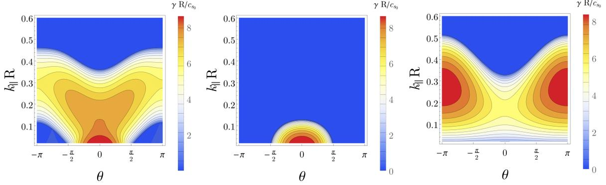
FIG. 4. Linear growth rate as a function of the poloidal angle,  $\theta$ , and of the parallel wavenumber normalized to the major radius  $k_{\parallel}R$ . From left to right: the solution of the full dispersion relation that couples inertial DW and BM, Eq. (8); the solution of Eq. (10) for the pure BM; and the solution of Eq. (11) for the pure DW.
