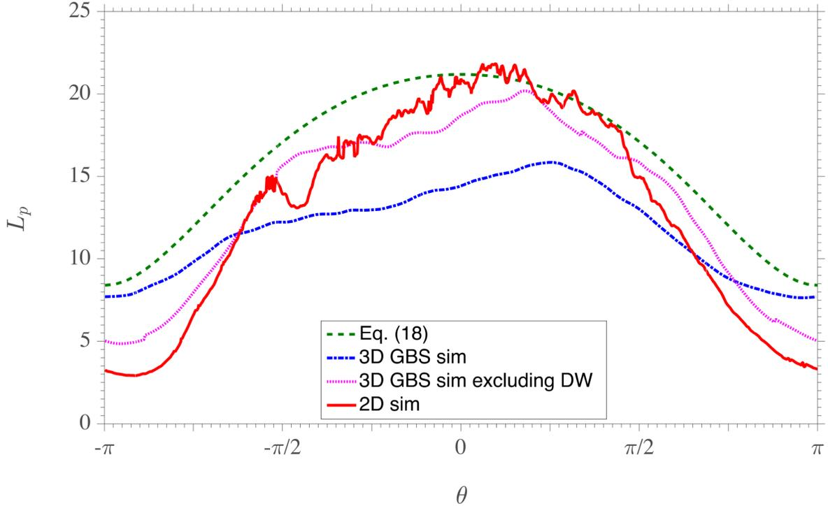
FIG. 3. The equilibrium pressure scale length,  $L_p$ , is plotted as a function of the poloidal angle,  $\theta$ , from an exponential fit in the radial direction of the type  $p/p_0 = e^{-x/L_p(\theta)}$  of the two- (red) and three-dimensional simulations, with (blue) and without (purple) DW, and the prediction from Eq. (18) (green).
