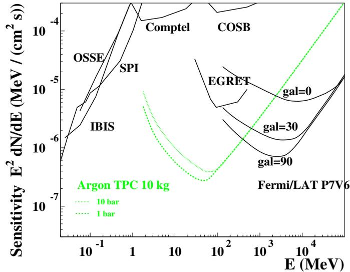
Figure 1: Differential sensitivity as a function of energy (argon-gas-based HARPO TPC, green) compared to the  $90^\circ$  galactic latitude performance of the *Fermi*-LAT [2] and of the Compton telescope COMPTEL [1]. Adapted from [6].
