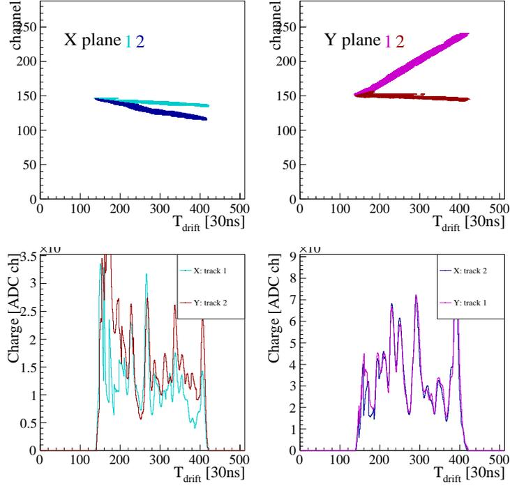
Figure 6: Procedure for matching the two projections of a vertex. Top: definition of the region associated to each of the two particles in the vertex. Middle: comparison of the charge profile (in  $Z$  direction) of  $X$ - $Y$  track combinations. The covariance of these distributions is used to select the best match.
