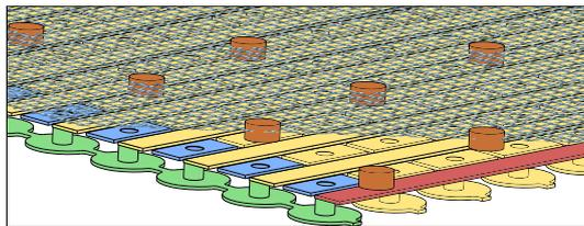
Figure 2: Detail of the micromegas and readout strips configuration.
