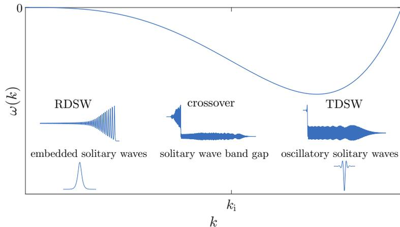
FIGURE 5. Non-convex Kawahara dispersion relation for  $\sigma = +1$  along with example numerical simulations for step initial data. The RDSW, crossover regime, and TDSW can be identified with properties of the dispersion curvature and the existence of solitary wave structures.
