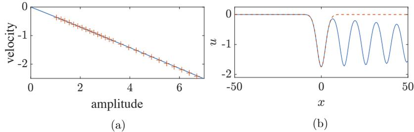
FIGURE 15. Comparison of DSW leading edge properties to Kawahara solitary waves. (a) Speed-amplitude relation of Kawahara solitary wave (solid) and DSW trailing edge (pluses) for  $\sigma = +1$ . (b) Overlay of numerically computed solitary wave with coincident velocity with the DSW trailing edge for  $\Delta = 1$ .
