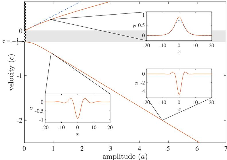
FIGURE 4. Solitary wave profiles and speed-amplitude relation for the Kawahara equation with  $\sigma = +1$  (solid) and KdV equation (dashed). The linear wave spectrum is denoted on the vertical axis by the thick black curve. The “band gap” where no solitary waves exist is the shaded region.
