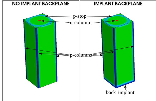
Figure 16: Net doping profile of the 3D-Si single sided without implant on the backside (left) and with implant on the backside (right).
