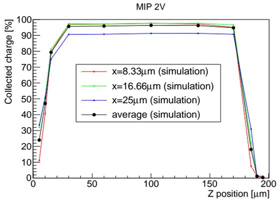
Figure 13: Simulation of a MIP impinging perpendicularly to the columns of a  $50\ \mu\text{m} \times 50\ \mu\text{m} \times 200\ \mu\text{m}$  detector biased at 2 V.
