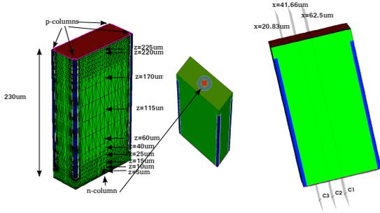
Figure 8:  $z$  positions of the simulated particles (left) and  $x$  planes (right).
