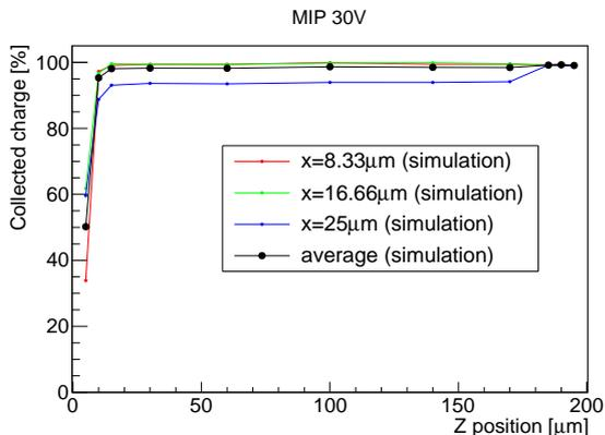
Figure 14: Simulation of a MIP impinging perpendicularly to the columns of a  $50\ \mu\text{m} \times 50\ \mu\text{m} \times 200\ \mu\text{m}$  detector biased at 30 V.
