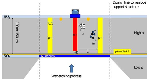
Figure 15: Scheme for 3D-Si single side detector.
