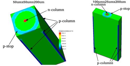
Figure 1: Simulated pixel cell for  $50\ \mu\text{m} \times 50\ \mu\text{m} \times 200\ \mu\text{m}$  (left) and  $100\ \mu\text{m} \times 25\ \mu\text{m} \times 200\ \mu\text{m}$  (right) geometry.
