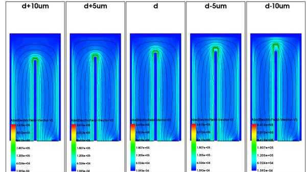
Figure 20: Cross sections of the electric field simulation for the 3D-Si single sided detectors with different depths of the columns with implant in the backplane. The electric field is at break-down voltage (circa 140 V), shown in fig. 22. The black lines are the equipotential lines.
