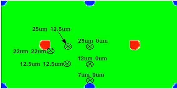
Figure 5: Collected charge for MIP in different positions for irradiated  $50\ \mu\text{m}\times 50\ \mu\text{m}\times 200\ \mu\text{m}$  sensor at  $2 \times 10^{16}\ \text{n}_{\text{eq}}\ \text{cm}^{-2}$ . The lower part of the figure shows the different positions of the MIP.
