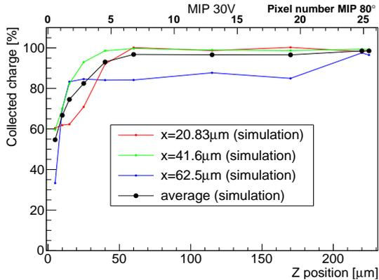
Figure 11: Simulation of MIP particles through different positions of the  $50\ \mu\text{m} \times 125\ \mu\text{m} \times 230\ \mu\text{m}$  pixel cell at 30 V. The upper axis corresponds to the pixel number of the experiment for large  $\eta$ , tilted  $80^\circ$  from the beam.
