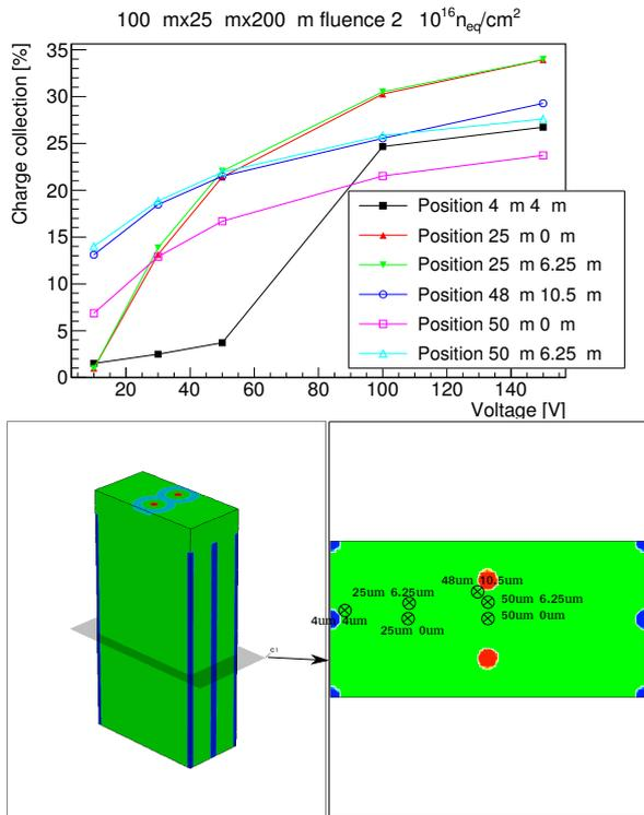
Figure 7: Collected charge for a MIP in different positions for an irradiated sensor at a fluence of  $2 \times 10^{16} n_{eq} cm^{-2}$ . The lower part of the figure shows a cross section of the two pixel cells with the different positions of the MIP.
