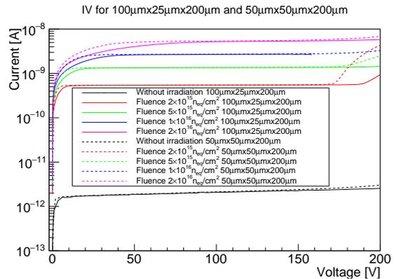
Figure 2: Current-voltage curves simulated for  $50\ \mu\text{m} \times 50\ \mu\text{m} \times 200\ \mu\text{m}$  and  $100\ \mu\text{m} \times 25\ \mu\text{m} \times 200\ \mu\text{m}$  single pixel cells at different fluences.
