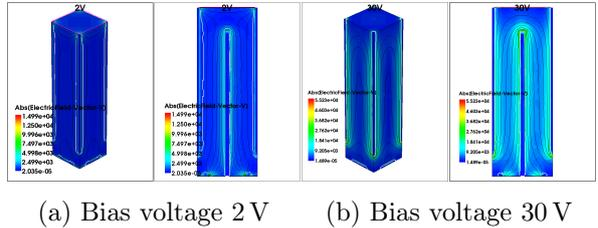
Figure 12: Simulation of the electric field for a  $50\ \mu\text{m} \times 50\ \mu\text{m} \times 200\ \mu\text{m}$  for two bias voltages, 2 V and 30 V. The left image is the pixel cell and the right image is the diagonal cross section of the pixel cell. The black lines are equipotential lines and the white line is the depletion region.
