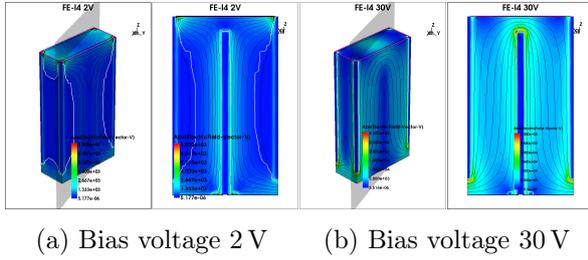
Figure 9: Simulation of the electric field for a  $50\ \mu\text{m} \times 125\ \mu\text{m} \times 230\ \mu\text{m}$  pixel cell for two bias voltages, 2 V and 30 V. The left image is the pixel cell and the right image is the diagonal cross section of the pixel cell. The black lines are equipotential lines and the white line is the depletion region.
