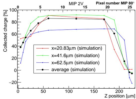
Figure 10: Simulation of MIP particles through different positions of the  $50\ \mu\text{m} \times 125\ \mu\text{m} \times 230\ \mu\text{m}$  pixel cell at 2 V. The upper axis corresponds to the pixel number of the experiment for large  $\eta$ , tilted  $80^\circ$  from the beam.
