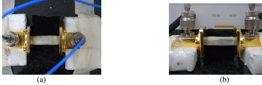
Fig.4. (a) Top view (b) Side view of the parallel plate waveguide experiment.
