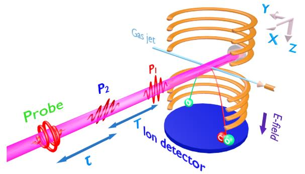
FIG. 1: **Experimental setup.** A supersonic gas jet of CO<sub>2</sub> molecules subject to a pair of polarization-skewed and time-delayed femtosecond laser pulses in an ultrahigh vacuum chamber of COLTRIMS is used to create molecular alignment echoes. By scanning the delay of an intense circularly polarized probe pulse, snapshots of the angular alignment of the molecular axis at various times are taken via Coulomb explosion.
