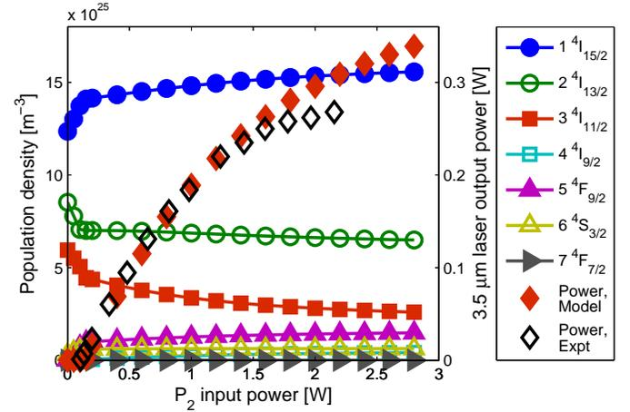
Fig. 10. Modeled populations of experiment H2014 by Henderson-Sapir *et al.* [6] as a function of  $P_2$  pump power. The populations are averaged over the length of the fiber at the end of a 20 ms simulation. The 3.47  $\mu\text{m}$  laser output power is plotted against the right axis to show the relation between laser output power and steady state populations.
