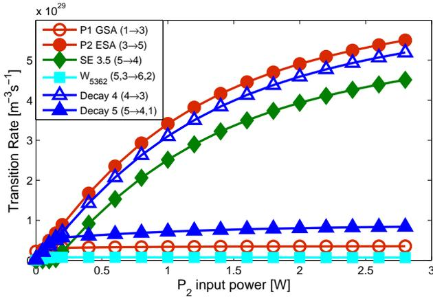
Fig. 12. Modeled transition rates of experiment H2014 by Henderson-Sapir *et al.* [6]. Rates are averaged over the length of the fiber and plotted as functions of incident  $P_2$  pump power. The transitions are pump absorption of  $P_1$  and  $P_2$  (P1 GSA and P2 ESA), stimulated emission (SE) of the 3.5  $\mu\text{m}$  laser, the cross relaxation process  $W_{5362}$ , and the decay rates from the lower (4) and upper (5) laser levels.
