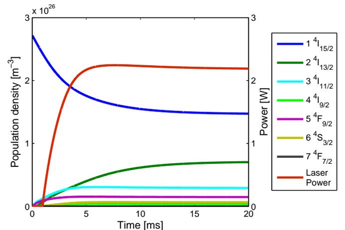
Fig. 4. Modeled atomic populations of experiment H2014 by Henderson-Sapir *et al.* [6]. The populations are calculated midway along the fiber in the case where pump  $P_1$  operates at 194 mW and  $P_2$  operates at 2 W CW. The intracavity 3.47  $\mu\text{m}$  laser power propagating in the '+' direction is plotted against the right axis.
