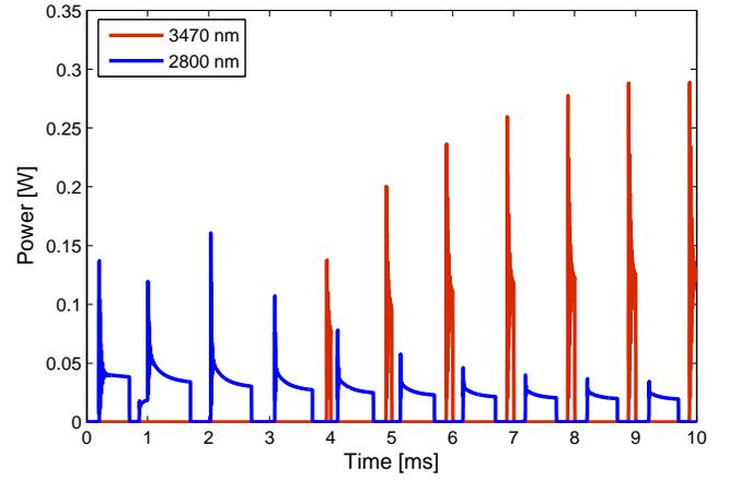
Fig. 6. Modeled intracavity laser power of experiment H2014 by Henderson-Sapir *et al.* [6], [30] in low power pulsed operation. The power is calculated midway along the fiber over a 10 ms simulation. Pump  $P_2$  operates at 200 mW with 300  $\mu\text{s}$  pulses at a repetition rate of 1 kHz. Lasers pulse alternately between wavelengths of 2.8  $\mu\text{m}$  and 3.47  $\mu\text{m}$ .
