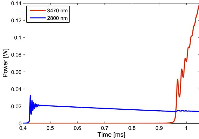
Fig. 5. Modeled intracavity laser power of experiment H2014 by Henderson-Sapir *et al.* [6] immediately after threshold of the 2.8  $\mu\text{m}$  and 3.47  $\mu\text{m}$  lasers. The power is calculated midway along the fiber in the case where pump  $P_1$  operates at 194 mW and  $P_2$  operates at 2 W CW. The figure illustrates oscillatory behavior at each laser wavelength immediately after threshold. The powers plotted are for lasers propagating in the ‘+’ direction only.
