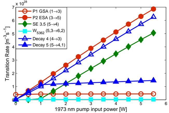
Fig. 14. Modeled transition rates of experiment H2016 by Henderson-Sapir *et al.* [7]. The rates are averaged over the length of the fiber and plotted as functions of incident  $P_2$  pump power. The transitions are pump absorption of  $P_1$  and  $P_2$  (P1 GSA and P2 ESA), stimulated emission (SE) of the 3.5  $\mu\text{m}$  laser, the cross relaxation process  $W_{5362}$ , and the decay rates of the lower (4) and upper (5) laser levels.
