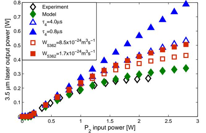
Fig. 11. Modeled CW 3.47  $\mu\text{m}$  laser output powers as functions of  $P_2$  pump power based on variations of experiment H2014 by Henderson-Sapir *et al.* [6]. The intrinsic lifetime  $\tau_4$  of the lower laser level  ${}^4I_{9/2}$  (4) and the cross relaxation parameter  $W_{5362}$  are reduced by factors of 2 and 10 separately.
