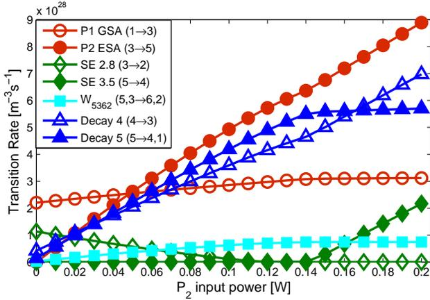
Fig. 13. Modeled transition rates of experiment H2014 by Henderson-Sapir *et al.* [6] around threshold. The rates are averaged over the length of the fiber and plotted as functions of incident  $P_2$  pump power. The transitions are pump absorption  $P_1$  and  $P_2$  (P1 GSA and P2 ESA), stimulated emission (SE) of the 2.8  $\mu\text{m}$  and 3.5  $\mu\text{m}$  lasers, the cross relaxation process  $W_{5362}$ , and the decay rates of the lower (4) and upper (5) laser levels.
