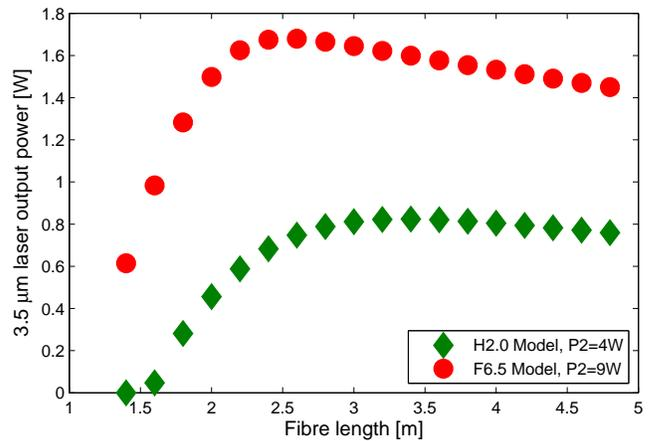
Fig. 15. Modeled laser output power as function of fiber length based on parameters from experiments H2016 by Henderson-Sapir *et al.* [7] (H2.0) and F2016 by Fortin *et al.* [10] (F6.5). The H2.0 simulation had  $P_2$  power fixed at 4 W and the F6.5 simulation had  $P_2$  power fixed at 9 W.
