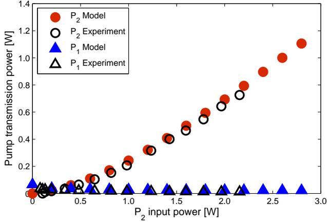
Fig. 8. Modeled CW pump transmission of experiment H2014 by Henderson-Sapir *et al.* [6] for the 985 nm ( $P_1$ ) and 1973 nm ( $P_2$ ) pumps. The incident power of  $P_1$  was held fixed at 194 mW while the incident power of  $P_2$  was varied.
