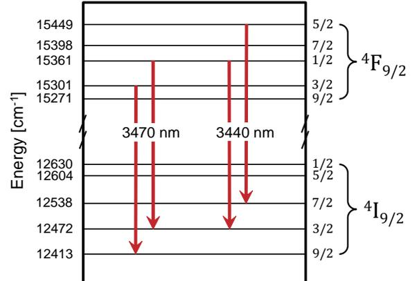
Fig. 3. Stark splitting in Er<sup>3+</sup>-doped ZBLAN and predicted laser transitions of lasers developed by Henderson-Sapir *et al.* [6], [7] (3470 nm) and Fortin *et al.* [10] (3440 nm). Each arrow connects a pair of Stark levels that correspond to the predicted transitions of the associated wavelengths. The energy data was sourced from Ref. [16] and the assignment order of Stark levels was sourced from Ref. [27].
