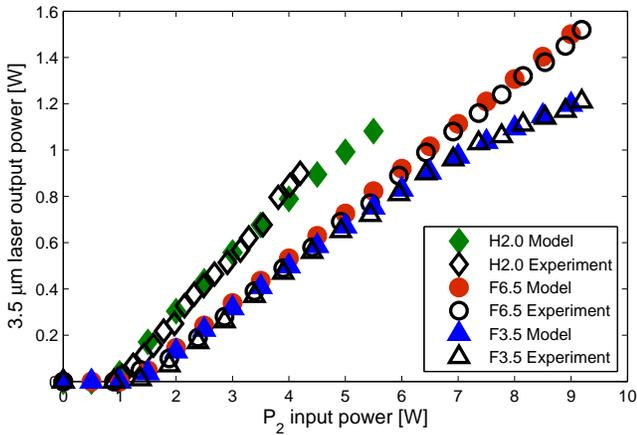
Fig. 9. Modeled 3.5  $\mu\text{m}$  laser output powers of experiments H2016 by Henderson-Sapir *et al.* [7] and F2016 by Fortin *et al.* [10]. ‘H2.0’ refers to the experiment H2016 in which  $P_1$  operated at 2.0 W. ‘F6.5’ and ‘F3.5’ refer to experiments F2016 in which  $P_1$  operated at 6.5 W and 3.5 W respectively.
