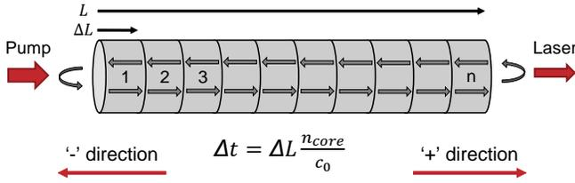
Fig. 2. Numerical iteration of photon propagation in a fiber divided into  $n$  length elements. Photons propagate in the ‘+’ or ‘-’ direction.  $n_{core}$  is the refractive index of the fiber core and  $c_0$  is the speed of light in a vacuum. The time step  $\Delta t$  is defined as the time required for light to traverse a single fiber element of length  $\Delta L = \frac{L}{n}$ .
