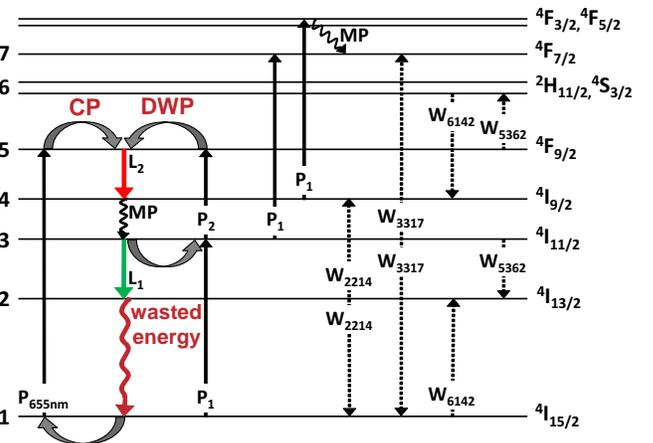
Fig. 1. The energy levels of erbium ions showing DWP transitions due to pump absorption of the first ( $P_1$ ) and second ( $P_2$ ) pumps, 2.8  $\mu\text{m}$  lasing ( $L_1$ ), 3.5  $\mu\text{m}$  lasing ( $L_2$ ), and energy transfer processes  $W_{ijk1}$ . A comparison between conventional pumping (CP) and dual-wavelength pumping (DWP) techniques is illustrated on the left. Two important multi-phonon (MP) decay processes are illustrated while other decay processes are omitted for brevity.
