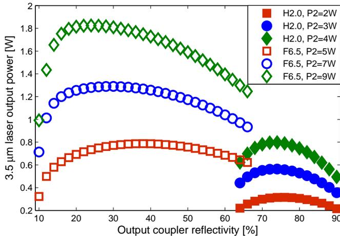
Fig. 16. Modeled laser output power as a function of output coupler reflectivity based on parameters from experiments H2016 by Henderson-Sapir *et al.* [7] (H2.0) and Fortin *et al.* [10] (F6.5). The H2.0 simulation had the power of  $P_2$  fixed at 4, 3, and 2 W. The F6.5 simulation had the power of  $P_2$  fixed at 9, 7, and 5 W.
