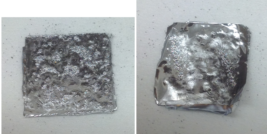
Figure 5. Left: sample with only 1 sheet of aluminum foil, which failed to extrude into foam. Right: sample with only 1 sheet of RBF but 2 sheets of aluminum foil, for which aluminum did not melt completely. Compare with Fig. 4, which demonstrates successful bonding.
