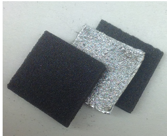
Figure 4. Mechanically-separated stack of carbon foam (top and bottom layers) and aluminum foil plus RBF (center) after bonding. The center piece is composed of 2 sheets of aluminum foil, 2 sheets of RBF, and another 2 sheets of aluminum foil all fused together by the RBF. The rough texture of the aluminum foil is caused by hundreds of branching extrusions which locked into the carbon foam.
