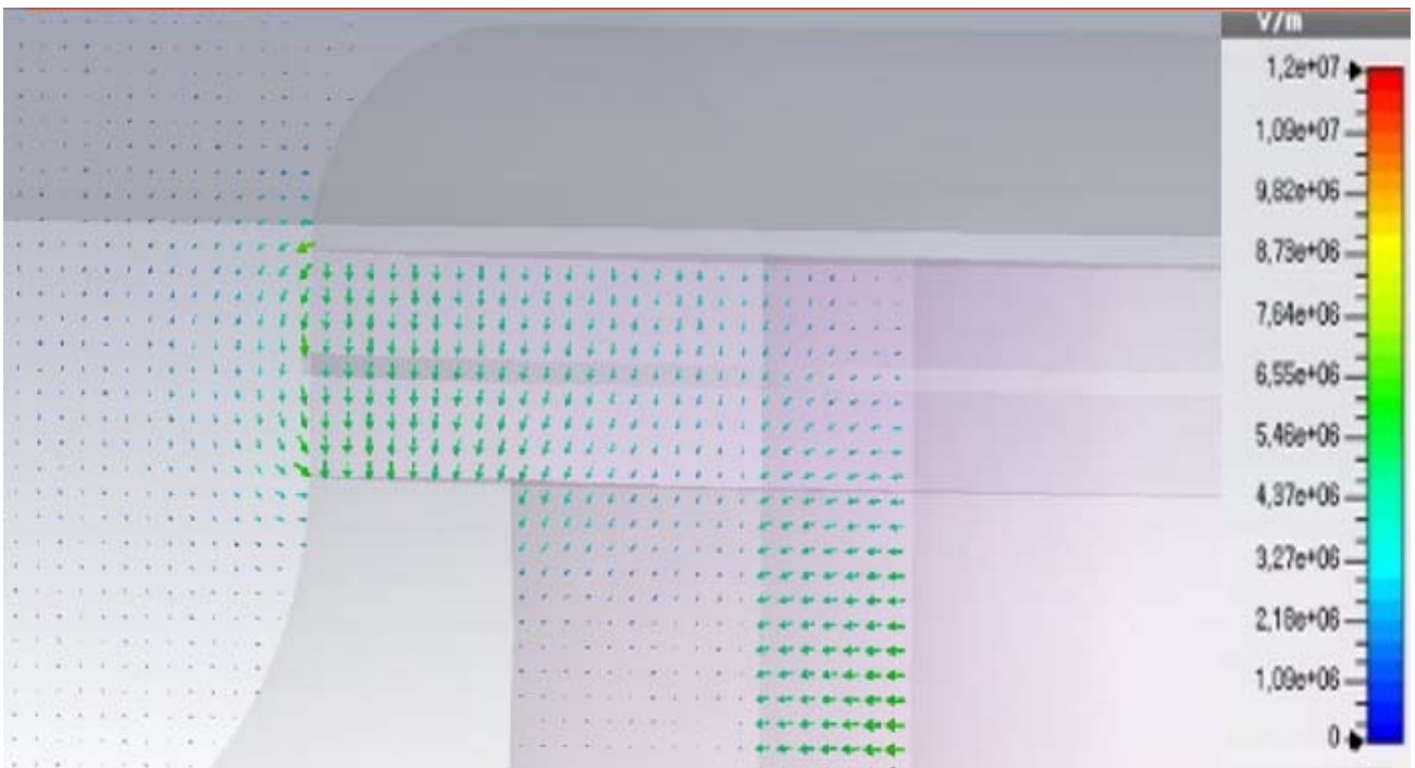
(a) The electric field of planar-convex (circular trigger pin and convex trigger electrode).
