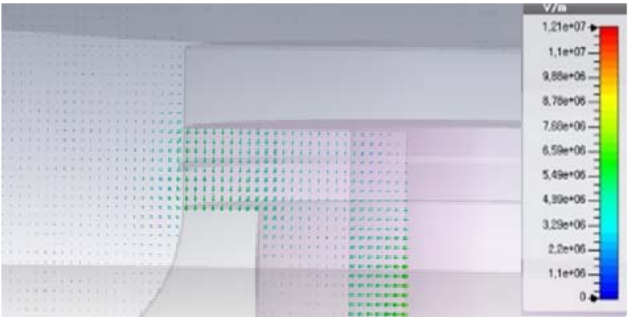
(a) The electric field of planar-convex (planar trigger pin and convex trigger electrode).
