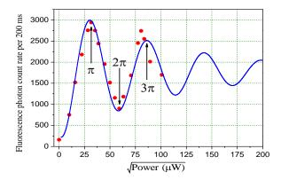
FIG. 6 Fluorescence photon count rate (red dots) as a function of the square root of the pulse laser power. The laser pulse duration is fixed at 5 ns, with a repetition rate of 10 MHz. The blue solid line is a theoretical curve based on a simple two-level model. The  $\pi$  pulsed laser power is  $\sim 1.25$  mW with pulse laser beam's waist:  $\sim 12$   $\mu$ m.
