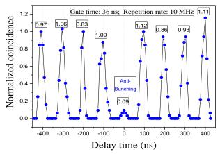
FIG. 7 Second-order intensity correlations of the single-photon source with background subtraction. Black dots are experimental data with 8 ns time bin. The absence of a peak at zero delay shows that the source is emitting single photons. Experimental parameters: pulse duration: 5 ns, repetition rate: 10 MHz, pulse laser beam's power:  $\sim 1.25$  mW, pulse laser beam's waist:  $\sim 12$   $\mu m$ ,  $I_{cool} = 10I_{sat}$ , PGC time: 690  $\mu s$ .
