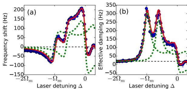
Figure 3. (color online) Optomechanical interaction for a polarization non-degenerate cavity. Blue points are extracted from the Lorentzian fit to the mechanical resonance. Red is a simultaneous fit of the data with four free parameters: optical linewidth, optical splitting and input laser power for both modes. Green shows the contribution of the individual modes. (a) Mechanical frequency shift (b) Effective mechanical damping.
