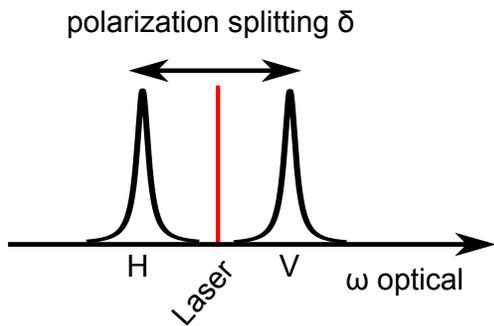
Figure 1. Polarization splitting leads to two distinct optical modes when the splitting  $\delta$  is larger than the cavity linewidth  $\kappa$ . H and V denote the different polarization and corresponding cavity mode.
