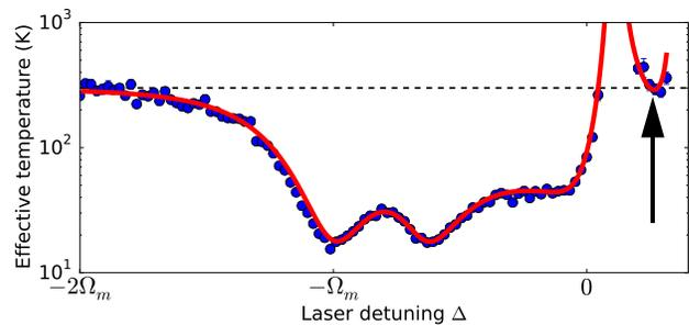
Figure 4. (color online) Effective temperature as a function of laser detuning. The arrow indicates the point where the contribution from both modes precisely cancel each other, leading to an effective temperature equal to the bath temperature.
