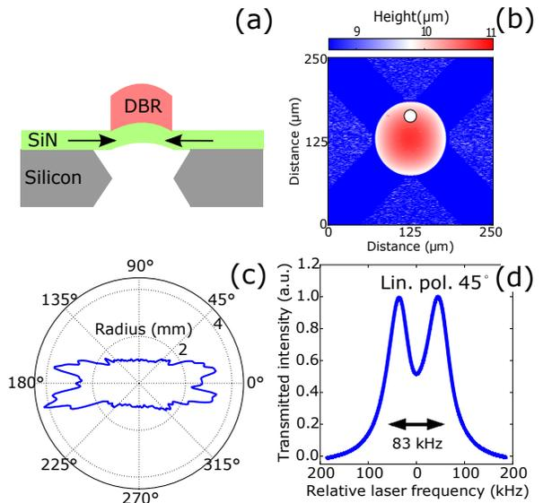
Figure 2. (a) Compressive stress in the DBR layers causes the mirror to buckle. (b) Optical profiling with a confocal microscope reveals a concave mirror surface. (c) Local radius of curvature as function of angle obtained for the off center location indicated with the white dot in (a). (d) Demonstration of mode splitting for an off axis aligned cavity by monitoring the transmitted intensity when the laser frequency is varied.
