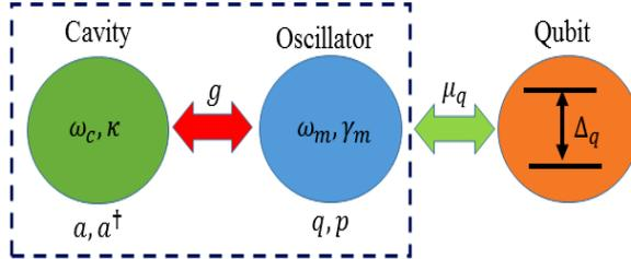
Figure 1: (Color online) Schematic diagram of the cavity optomechanical system which consists of an optical cavity with frequency  $\omega_c$  coupled to a mechanical mirror of frequency  $\omega_m$ , via radiation pressure. Furthermore, we consider the mechanical mirror to be perturbatively coupled to an auxiliary qubit.
