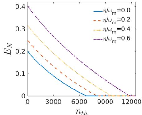
Figure 4: (Color online) Plot of logarithmic negativity  $E_N$  as a function of the mean thermal phonon number  $n_{th}$ . Here, the effective cavity detuning and optomechanical coupling strength are respectively fixed at  $\Delta/\omega_m = 0.5$  and  $G/\omega_m = 0.6$ , with all the other parameters same as in Fig. 2.
