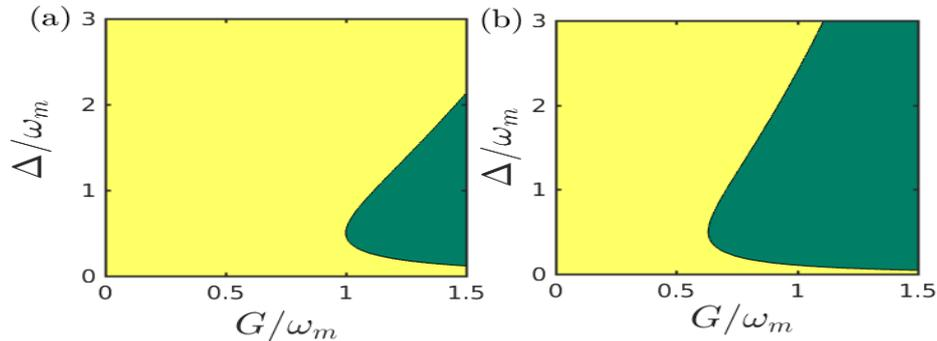
Figure 2: (Color online) Stable (yellow) and unstable (green) region of the optomechanical system in the  $(G/\omega_m, \Delta/\omega_m)$  plane, respectively for (a)  $\eta/\omega_m = 0$  and (b)  $\eta/\omega_m = 0.6$ . The other parameters are chosen to be  $\omega_m/(2\pi) = 10$  MHz,  $Q = 10^5$ ,  $\kappa/(2\pi) = 5$  MHz and  $T_0 = 0.6$  K.
