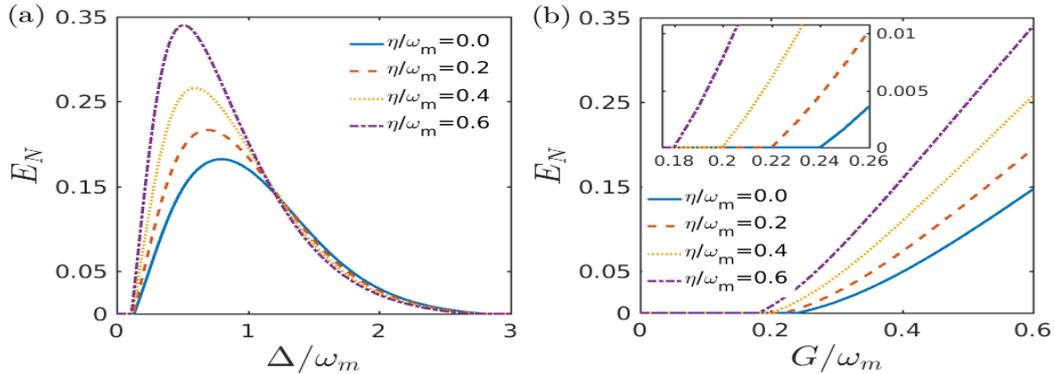
Figure 3: (Color online) Plot of logarithmic negativity  $E_N$  as a function of (a) normalized detuning  $\Delta/\omega_m$  for a fixed coupling strength  $G/\omega_m = 0.6$  and (b) dimensionless effective optomechanical coupling strength  $G/\omega_m$  at a fixed detuning  $\Delta/\omega_m = 0.5$ , with all the other parameters same as in Fig. 2.
