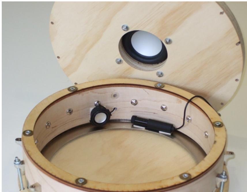
FIG. 11. plywood heads, speakers, & mic
