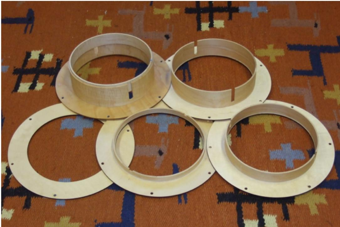
FIG. 13. internal resonators of various and variable heights
