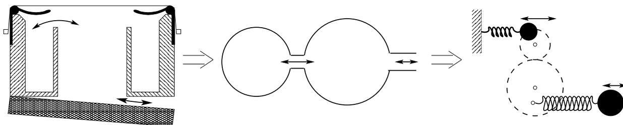
FIG. 4. The double-Helmholtz interpretation of the internal resonator
