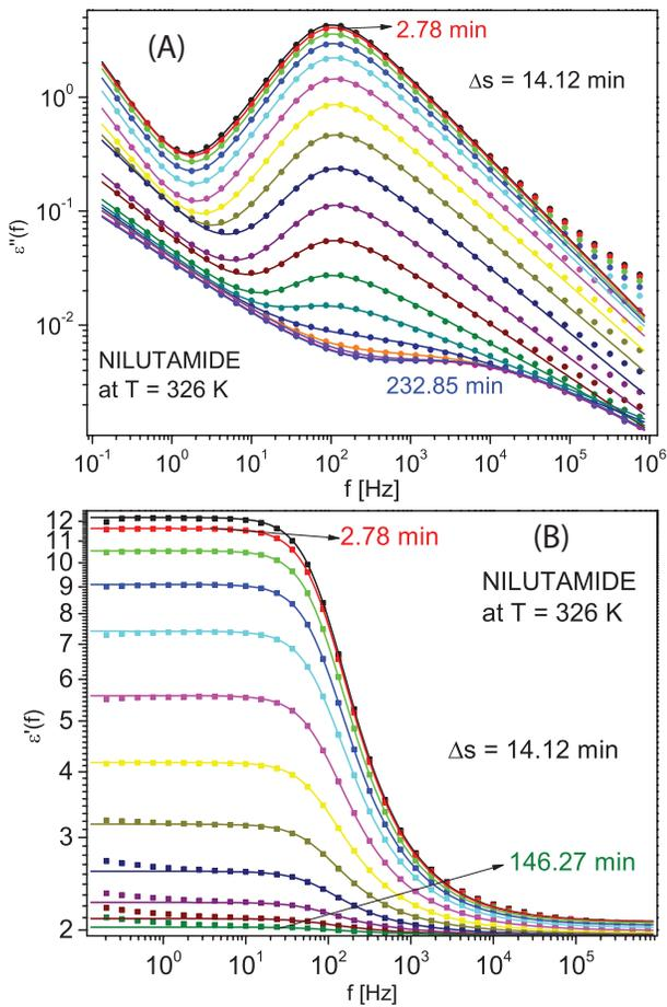
FIG. 7. (A). Imaginary and (B). real part of permittivity at temperature 326 K for various time. The dielectric data at initial, 2.78 min. and time interval of 14.12 min. are shown in the figure.
