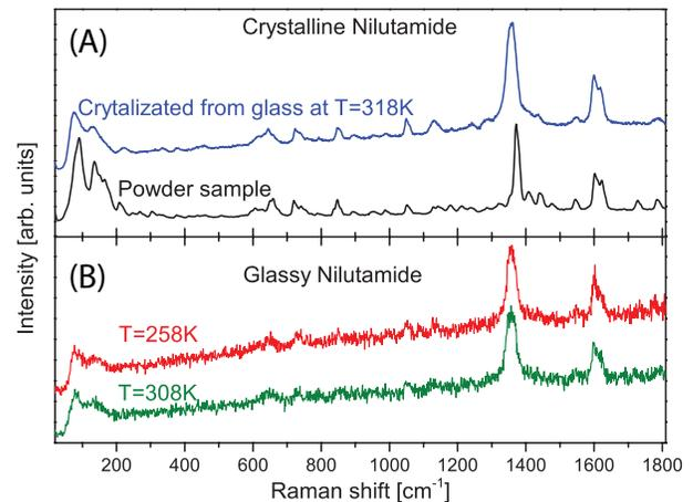
FIG. 2. (A). Raman spectra of nilutamide in crystalline (powder) and recrystallized form (B). Raman spectra of glassy form of nilutamide at two typical temperatures.
