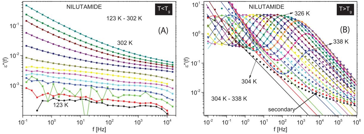
FIG. 3. (A). The dielectric loss data below  $T_g$  do not show well defined secondary processes. (B). The dielectric loss data above  $T_g$  structural  $\alpha$  relaxation process, excess wing like secondary process and dc conductivity due to translational motion of ions. The dielectric loss data are fitted with  $\sigma_{dc}$  and HN function for the  $\alpha$  relaxation process.
