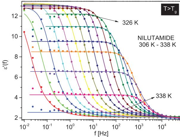
FIG. 4. Real part of dielectric permittivity at temperature above  $T_g$ . Nilutamide show a dramatic change in dielectric strength above the temperature 326 K, as an indication of crystallization of the sample.
