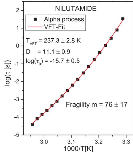
FIG. 5. The structural relaxation,  $\alpha$ -process of nilutamide shows non-Arrhenius behaviour and follows Vogel-Fulcher-Tammann (VFT) equation.
