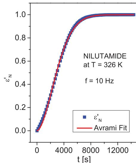
FIG. 8. Crystallization fraction as obtained from Eq.6 for the dielectric data at 10 Hz, of the crystallizing nilutamide at temperature of 326 K.
