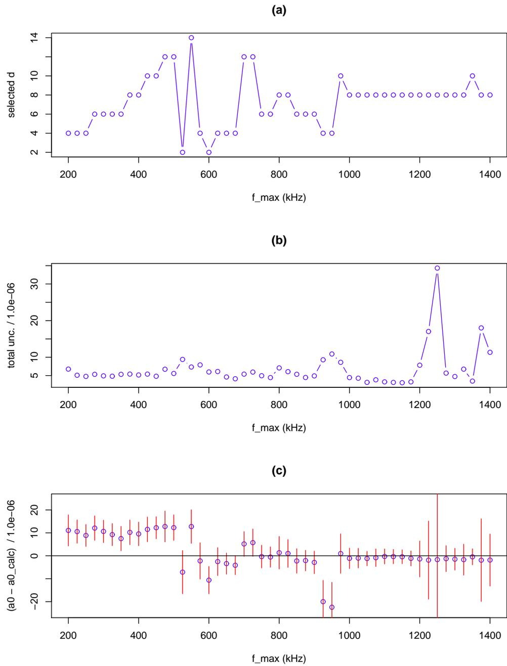
**Figure 5.** Simulated data (realization 2). (a) Estimated polynomial complexity parameter  $d$ . (b) Estimated total uncertainty  $\hat{\sigma}_{\text{tot}}$ . (c) Estimated  $a_0 - a_{0,\text{calc}}$  and approximate 68 % coverage interval. The true value of  $a_0 - a_{0,\text{calc}}$  is 0.
