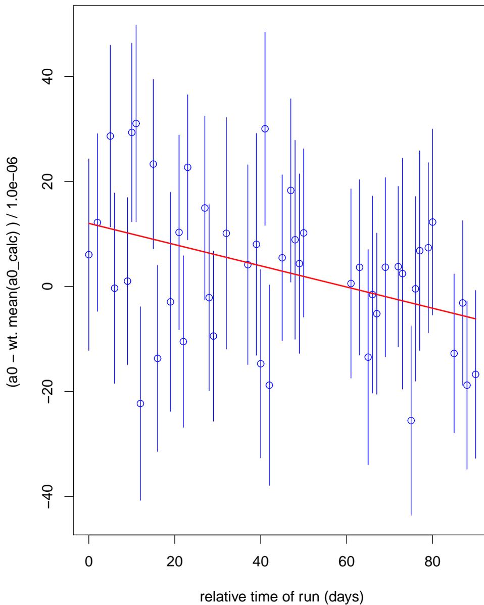
**Figure 8.** From the corrected ratio spectrum (Eq. 7), we estimate  $a_0 - \bar{a}_{0,\text{calc}}$  for each run by fitting a  $d = 8$  ratio spectrum model by the method of Least Squares. The half-widths of the intervals are asymptotic uncertainties determined by the Least Squares method. The fitting bandwidth is  $f_{\text{max}} = 1250$  kHz.
