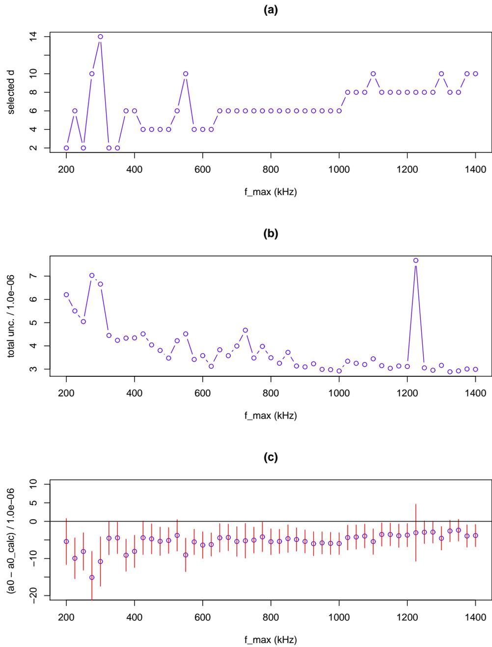
**Figure 6.** Simulated data (realization 3). (a) Estimated polynomial complexity parameter  $d$ . (b) Estimated total uncertainty  $\hat{\sigma}_{\text{tot}}$ . (c) Estimated  $a_0 - a_{0,\text{calc}}$  and approximate 68 % coverage interval. The true value of  $a_0 - a_{0,\text{calc}}$  is 0.
